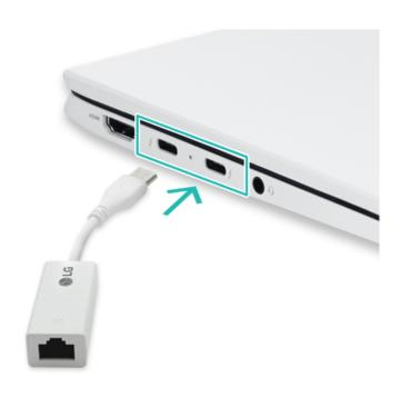
2 Connect the wired LAN cable to the LAN port.
