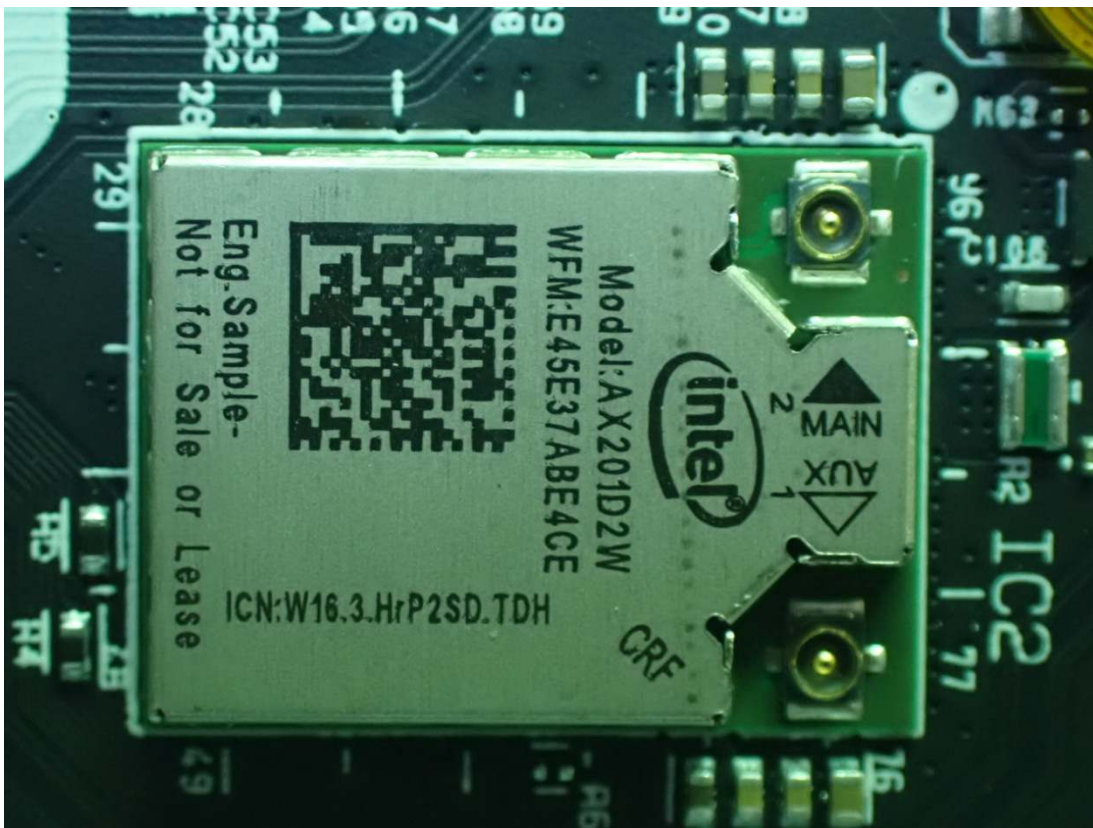
Figure 57 WLAN Combo Card, Front View
