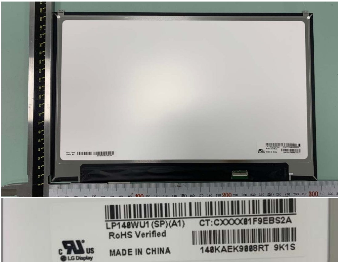
Figure 63 LCD Panel, Back / Label View
