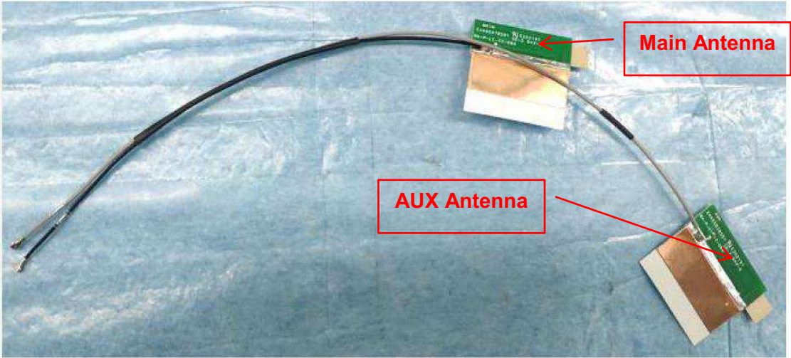
Figure 29 Antenna View, Front View
