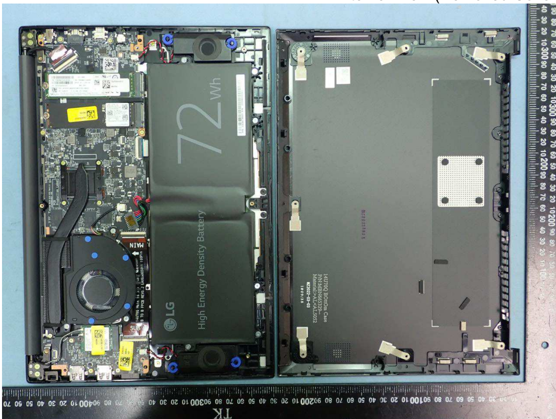
Figure 8 Internal View (Removed Cover)
