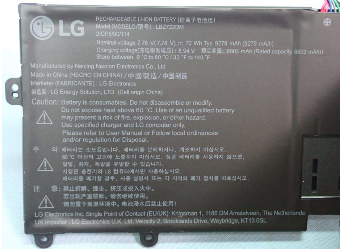
Figure 13 Battery Pack, Label View
