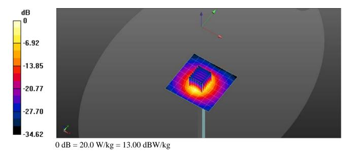
Frequency: 5200 MHz; Duty Cycle: 1:1; Room Ambient Temperature: 23.0°C; Liquid Temperature: 22.0°C Medium parameters used: f = 5200 MHz;  $\sigma$  = 4.458 S/m;  $\epsilon_r$  = 37.383;  $\rho$  = 1000 kg/m<sup>3</sup> DASY5 Configuration:
