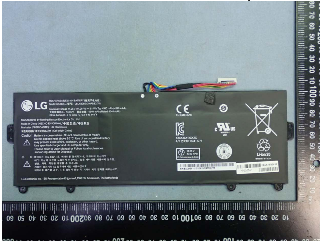
Figure 24 Battery Pack, Front View
