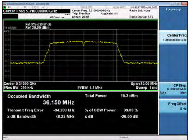
802.11n_HT40 UNII 3 BAND 26dB Bandwidth (CH 159)
