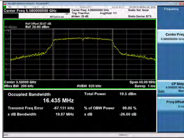
802.11a UNII 2C BAND 26dB Bandwidth (CH116)
