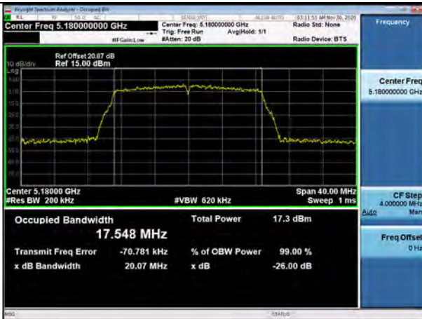
802.11n_HT20 UNII 2C BAND 26dB Bandwidth(CH 116)
