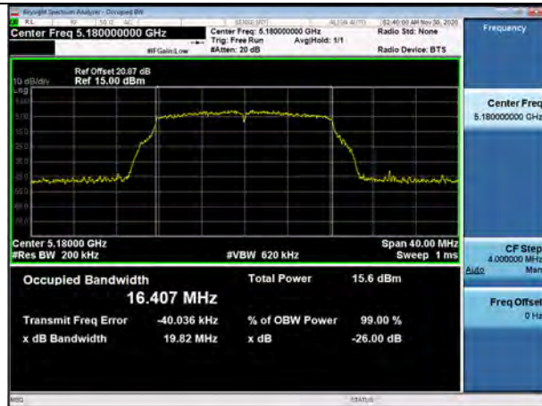
802.11a UNII 2C BAND 26dB Bandwidth (CH116)
