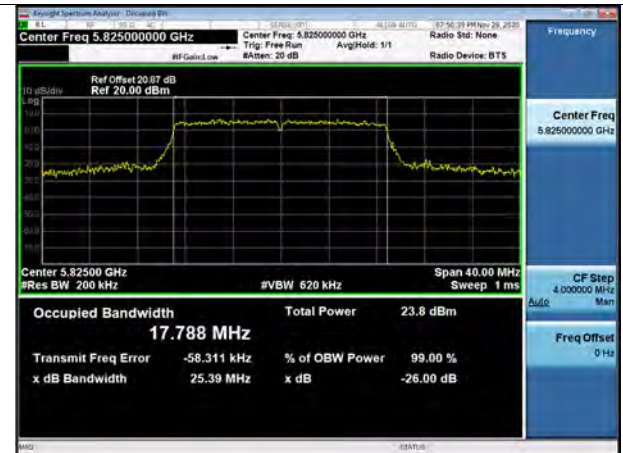
802.11ac_VHT20 UNII 3 BAND 26dB Bandwidth(CH 165)
