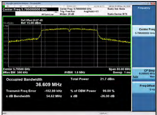
802.11n_HT40 UNII 3 BAND 26dB Bandwidth (CH 159)
