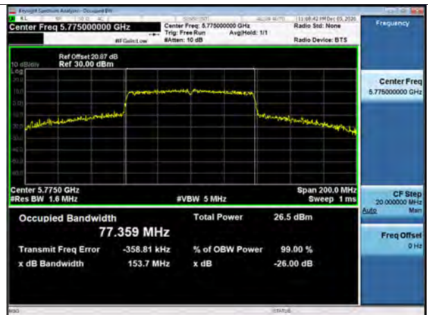
802.11ac_VHT80 UNII 3 BAND 26dB Bandwidth (CH 155)
