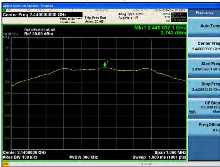
Power Spectral Density (Mid-CH 19)
