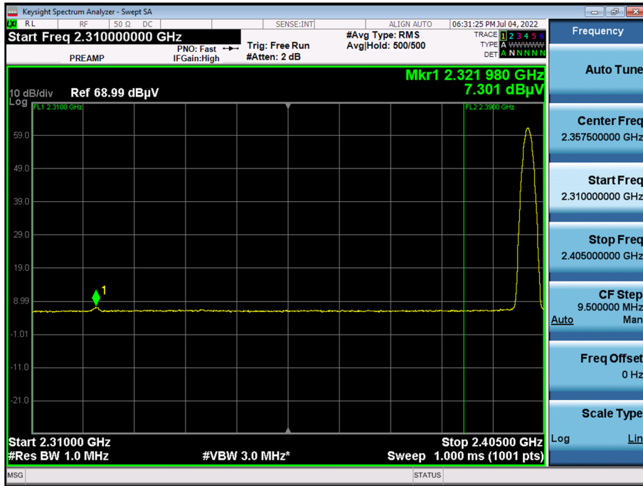
[Radiated Restricted Band Edges plot - Average Result]
