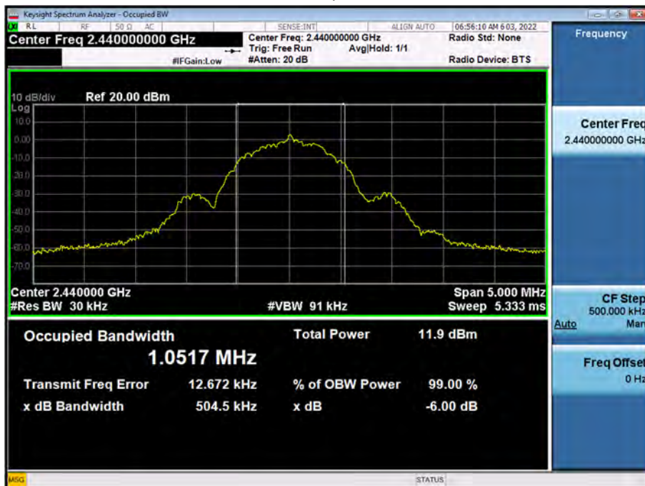
99 % Bandwidth plot (Mid-CH 19)
