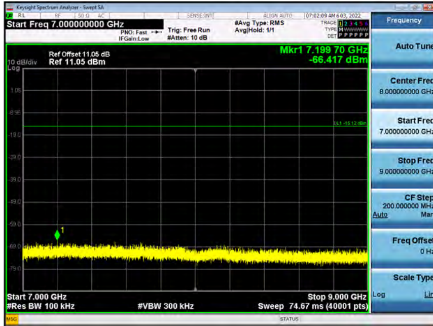
Conducted Spurious Emission (Mid-CH 16)
