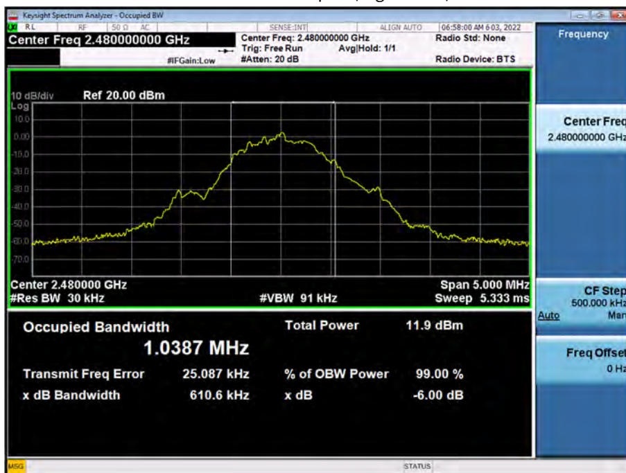
99 % Bandwidth plot (High-CH 39)
