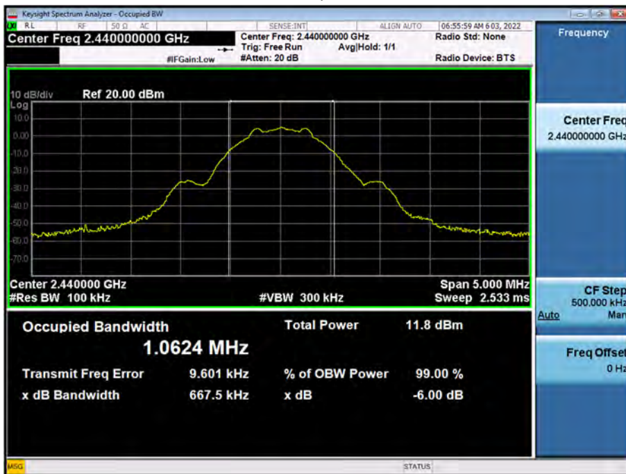
6 dB Bandwidth plot (Mid-CH 19)
