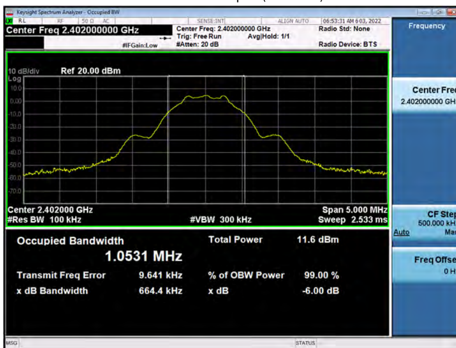
6 dB Bandwidth plot (Low-CH 0)
