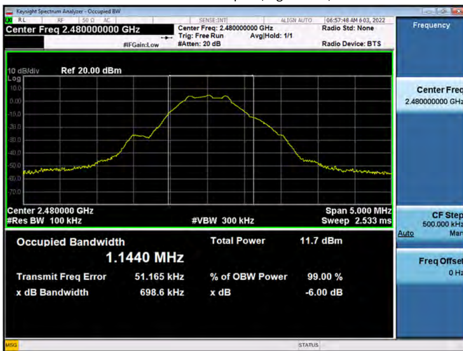
6 dB Bandwidth plot (High-CH 39)
