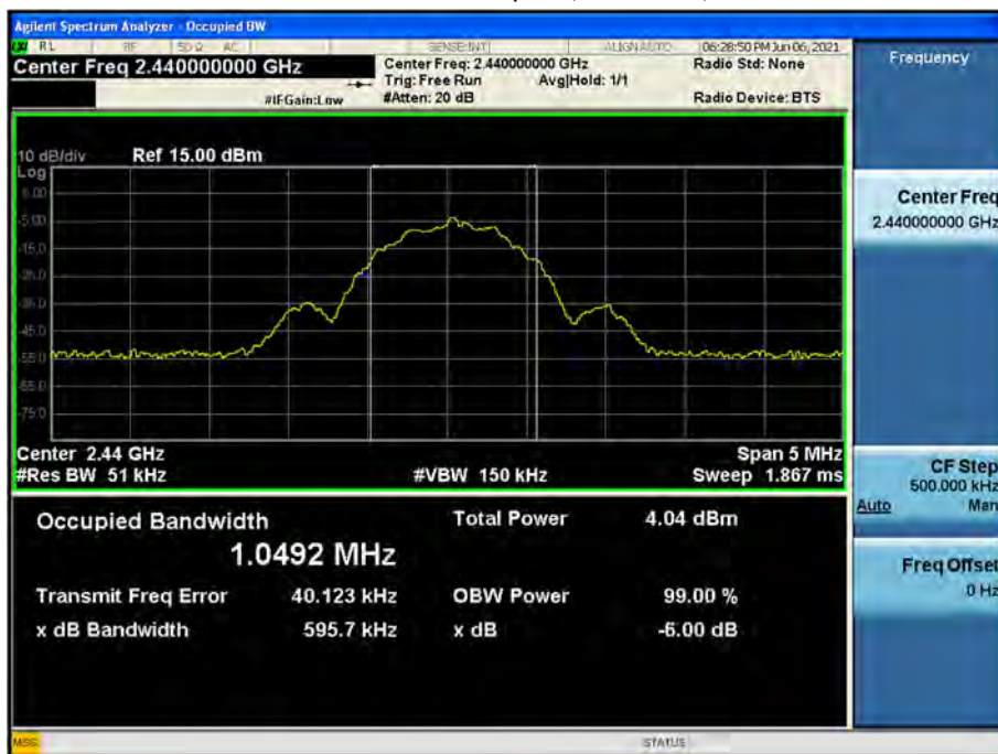
99 % Bandwidth plot (Mid-CH 19)
