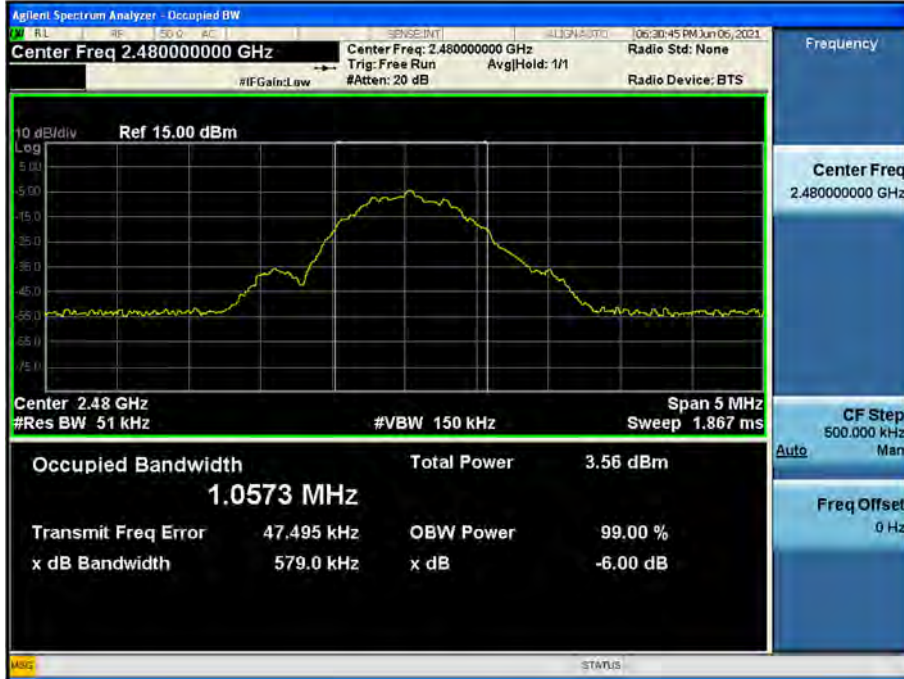
99 % Bandwidth plot (High-CH 39)
