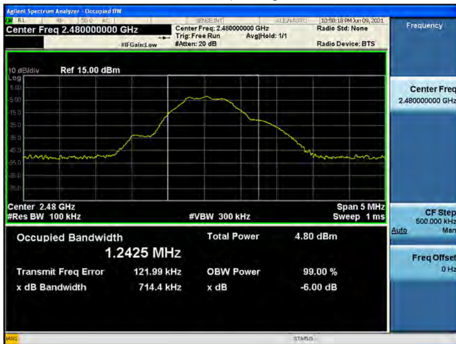
6 dB Bandwidth plot (High-CH 39)
