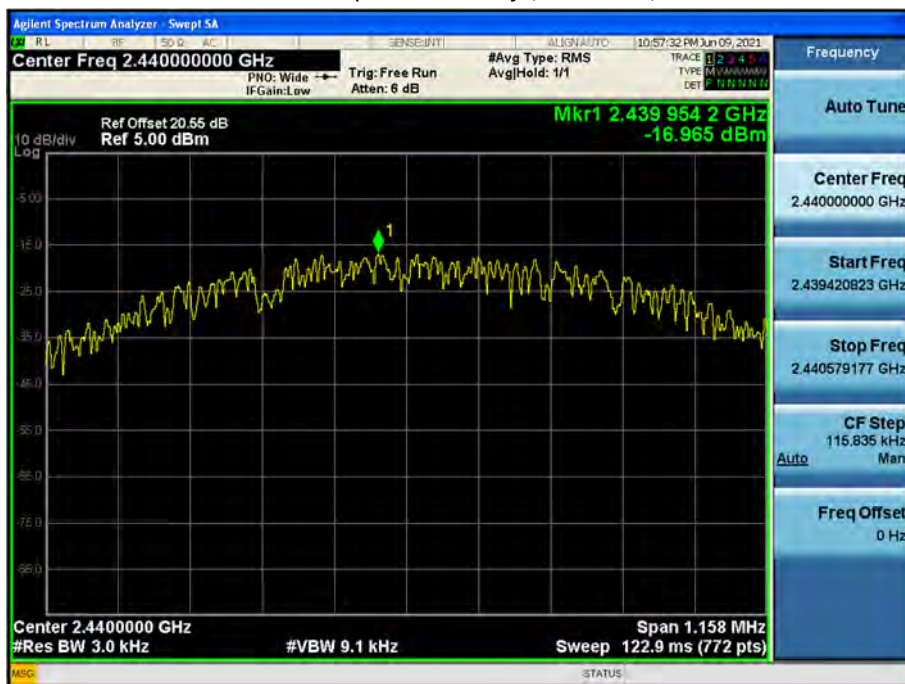
Power Spectral Density (Mid-CH 19)
