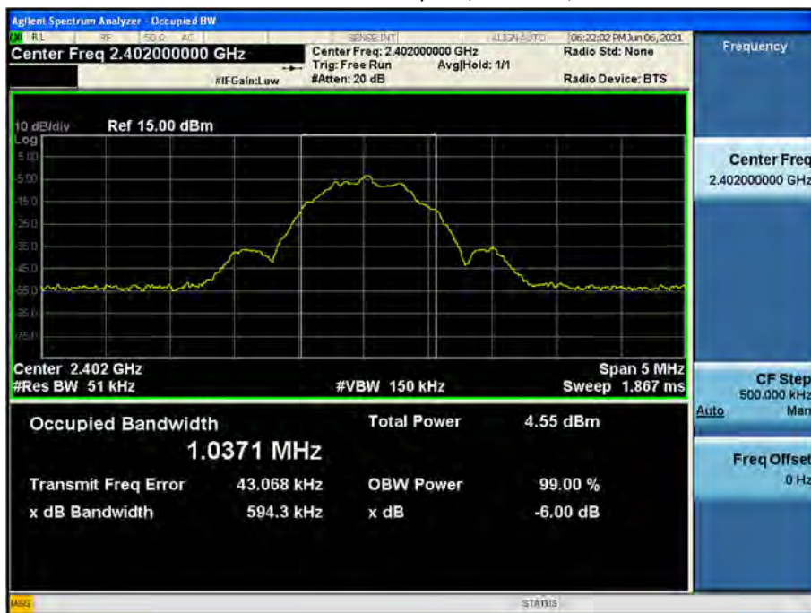
99 % Bandwidth plot (Low-CH 0)
