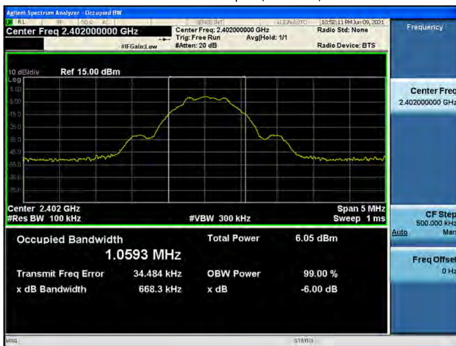
6 dB Bandwidth plot (Mid-CH 19)
