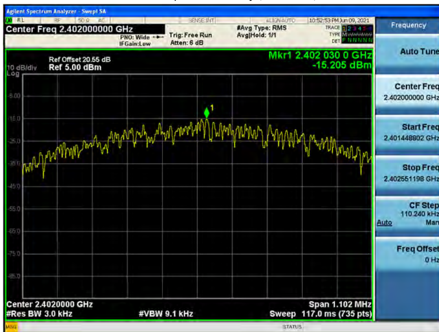
Power Spectral Density (Low-CH 0)
