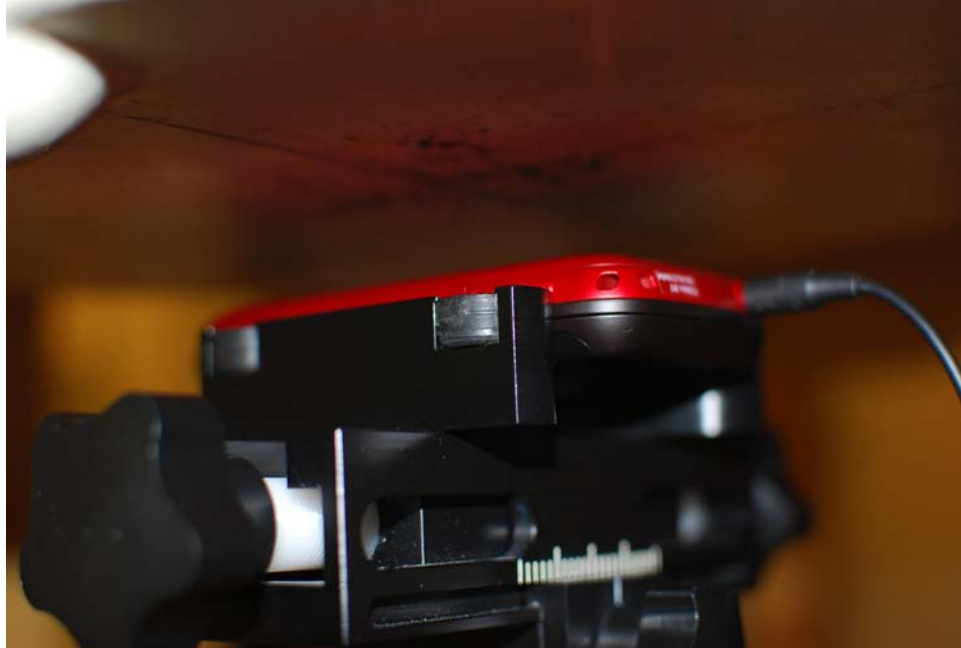
Figure 1-5 SAR Test Setup Photo 5 – Body Back Side
