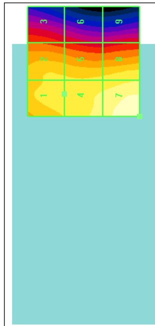
Figure 10-2 Sample H-field Scan Overlay (See Test Setup Photographs for actual WD overlay)
