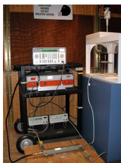
Figure A.0 Dipole Validation Test Setup
