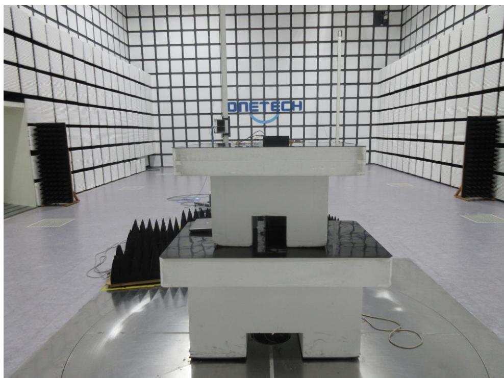
**- WLAN 5 GHz Radiated Emission Test (Below 1GHz)**
