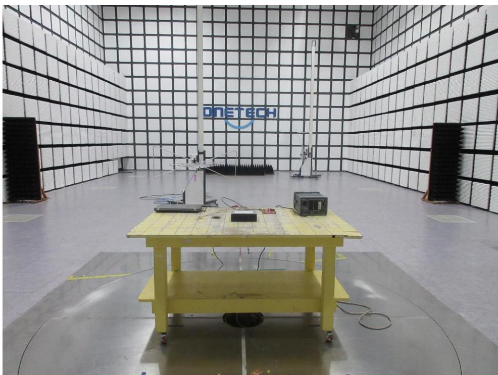
**- WLAN 2.4 GHz Radiated Emission Test (Above 1GHz)**
