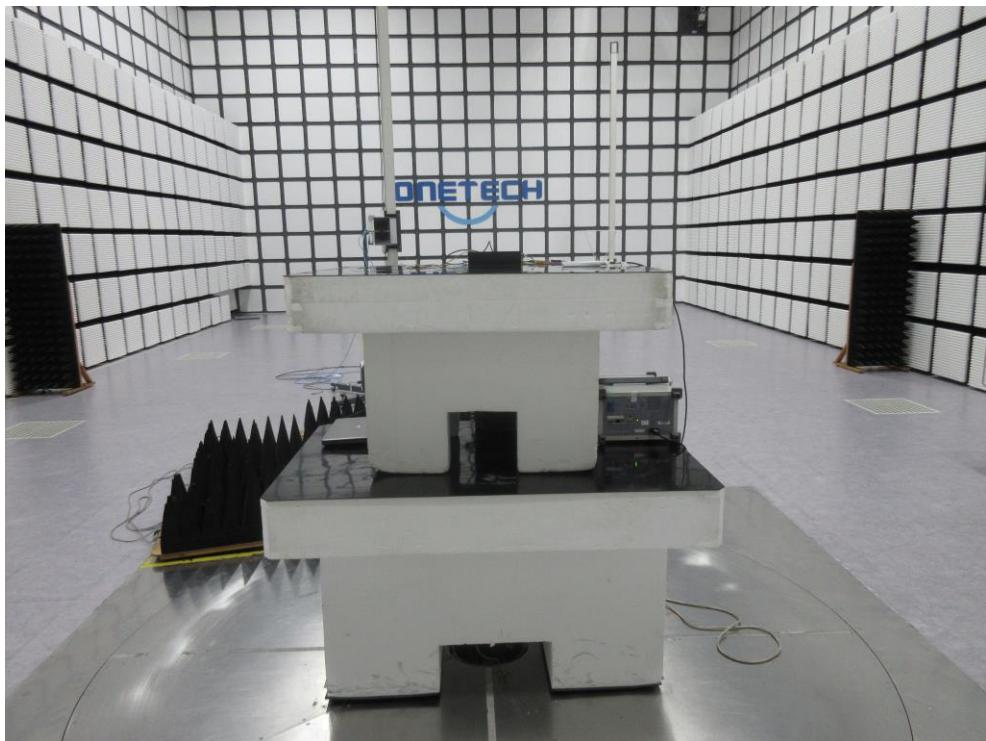
**- WLAN 2.4 GHz Radiated Emission Test (Below 1GHz)**
