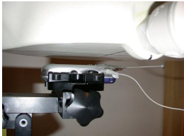
Figure 14.17 Body SAR Test Setup -- w/o Holster --
