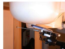
Figure 14.12 Right Head SAR Test Setup -- Ear / Tilt Position --
