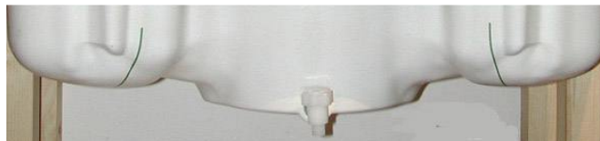
Figure 7.2 SAM Twin Phantom shell
