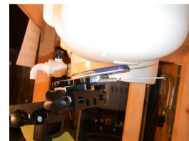
Figure 14.16 Left Head SAR Test Setup -- Ear / Tilt Position --
