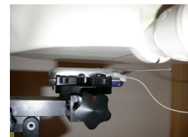
Figure 14.18 Body SAR Test Setup -- w/o Holster --
