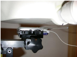
Figure 14.20 Body SAR Test Setup -- w/o Holster --
