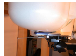
Figure 14.11 Right Head SAR Test Setup -- Cheek / Touch Position --
