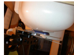
Figure 14.15 Left Head SAR Test Setup -- Cheek / Touch Position --
