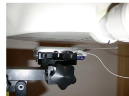
Figure 14.19 Body SAR Test Setup -- w/o Holster --
