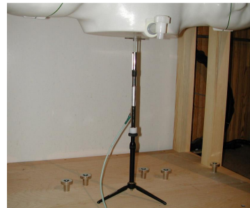
Figure 12.1 Dipole Validation Test Setup
