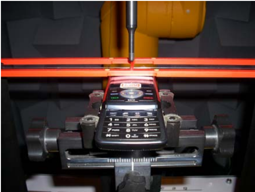
Figure 17-2 HAC Phantom Plane Alignment
