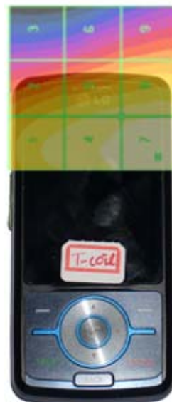
Figure 17-5 H-Field WD Scan overlay
