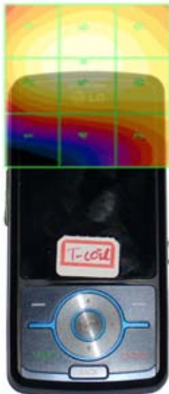
Figure 17-4 E-Field WD Scan overlay
