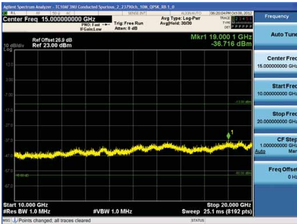
BAND 17. Conducted Spurious Plot_2 (23790ch_10MHz_QPSK_RB 1_0)
