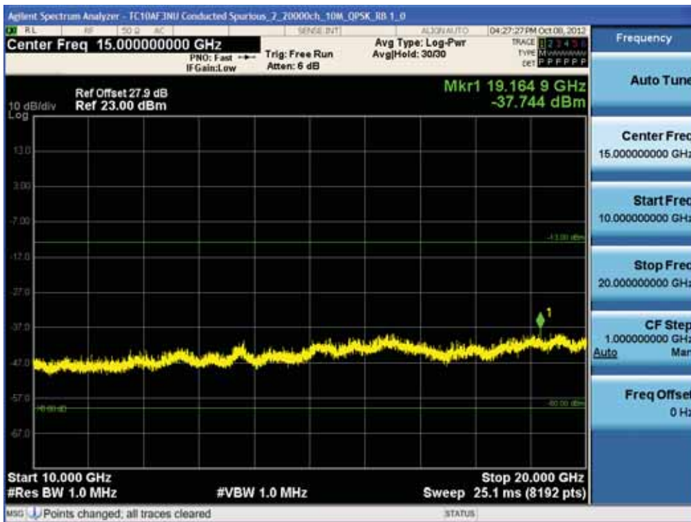
BAND . Conducted Spurious Plot_2 (20000ch_10MHz_QPSK_RB 1_0)
