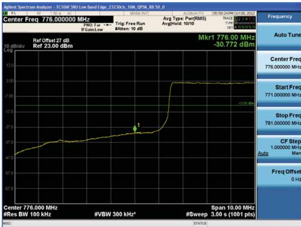
BAND 13. Low Band Edge Plot (23230ch_10MHz_QPSK_RB 50_0)
