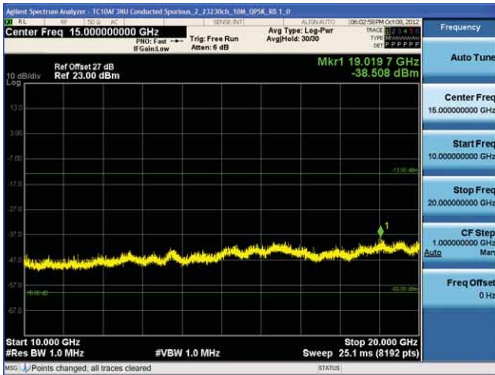
BAND 13. Conducted Spurious Plot_1 (23230ch_10MHz_QPSK_RB 1_0)
