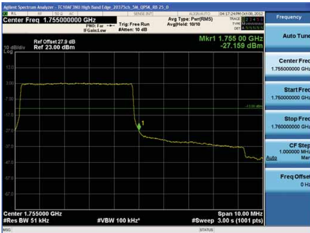
BAND 4. High Band Edge Plot (20375ch_5MHz_QPSK_RB 25_0)
