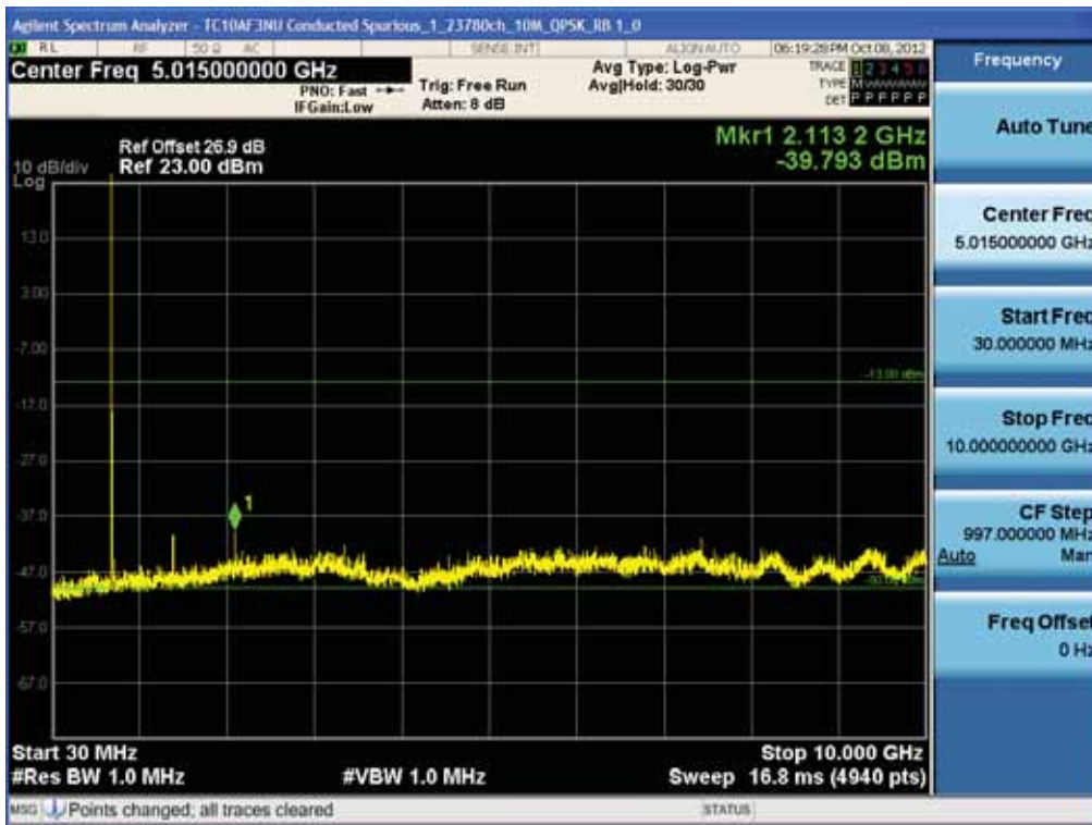
BAND 17. Conducted Spurious Plot_1 (23780ch_10MHz_QPSK_RB 1_0)
