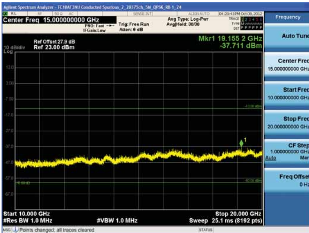
BAND 4 . Conducted Spurious Plot_2 (20375ch_5MHz_QPSK_RB 1_24)
