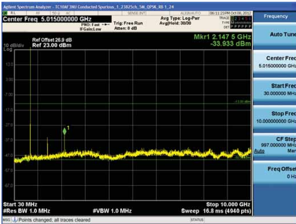
BAND 17. Conducted Spurious Plot_1 (23825ch_5MHz_QPSK_RB 1_24)
