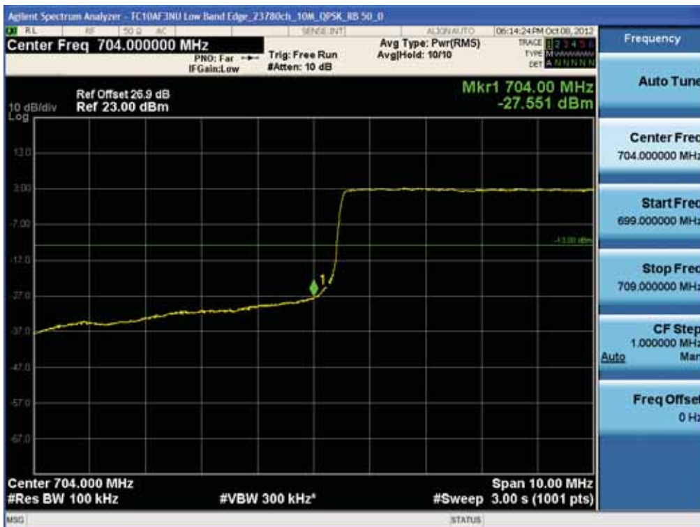
BAND 17. Low Band Edge Plot (23780ch_10MHz_QPSK_RB 50_0)
