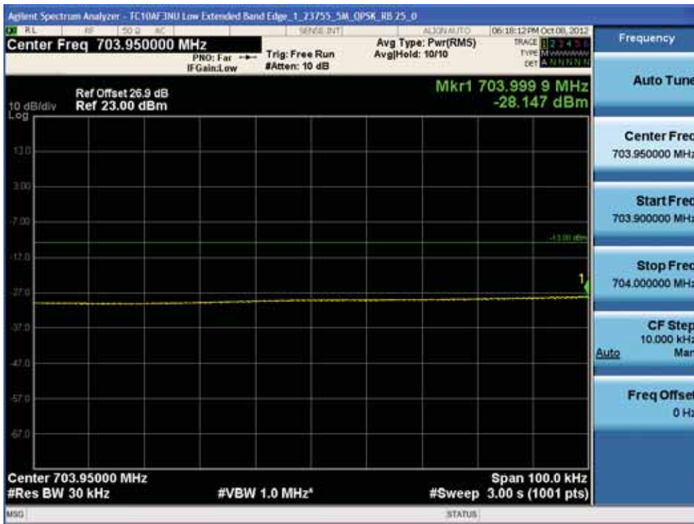
BAND 17. Low Extended Band Edge Plot _1 (23755ch_5MHz_QPSK_RB 25_0)
