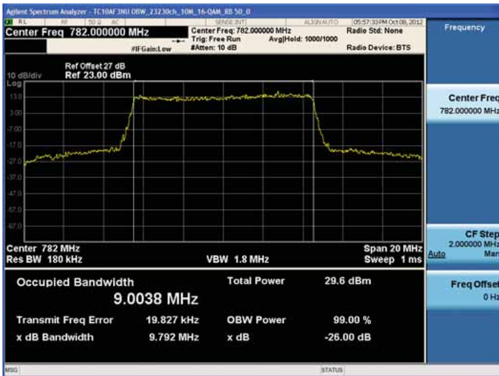
BAND 13. Occupied Bandwidth Plot (23230ch_10MHz_16-QAM_RB 50)
