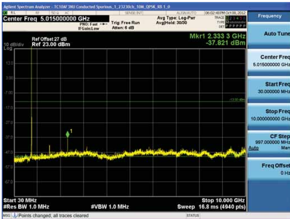
BAND 13. Conducted Spurious Plot_2 (23230ch_10MHz_QPSK_RB 1_0)
