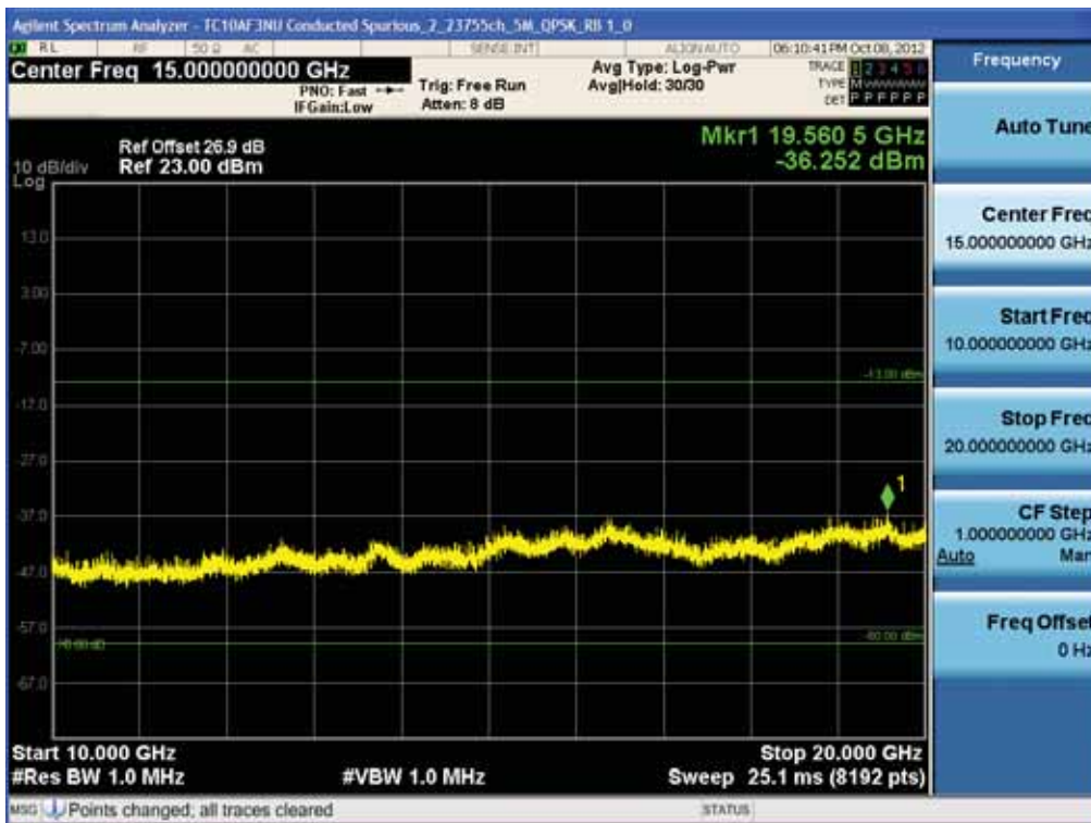
BAND 17. Conducted Spurious Plot_2 (23755ch_5MHz_QPSK_RB 1_0)
