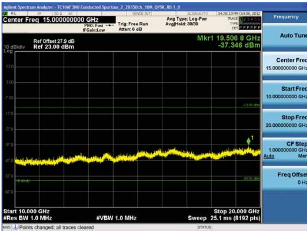
BAND 4. Conducted Spurious Plot_2 (20350ch_10MHz_QPSK_RB 1_0)
