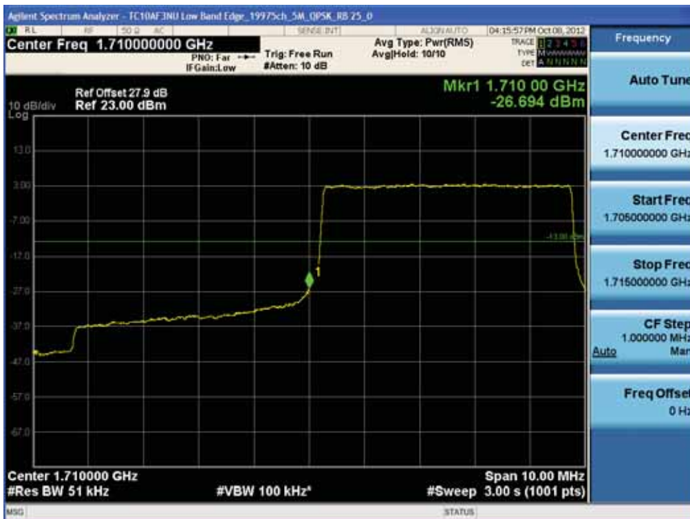
BAND 4. Low Band Edge Plot (19975ch_5MHz_QPSK_RB 25_0)
