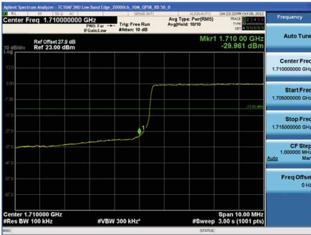
BAND 4. Low Band Edge Plot (20000ch_10MHz_QPSK_RB 50_0)
