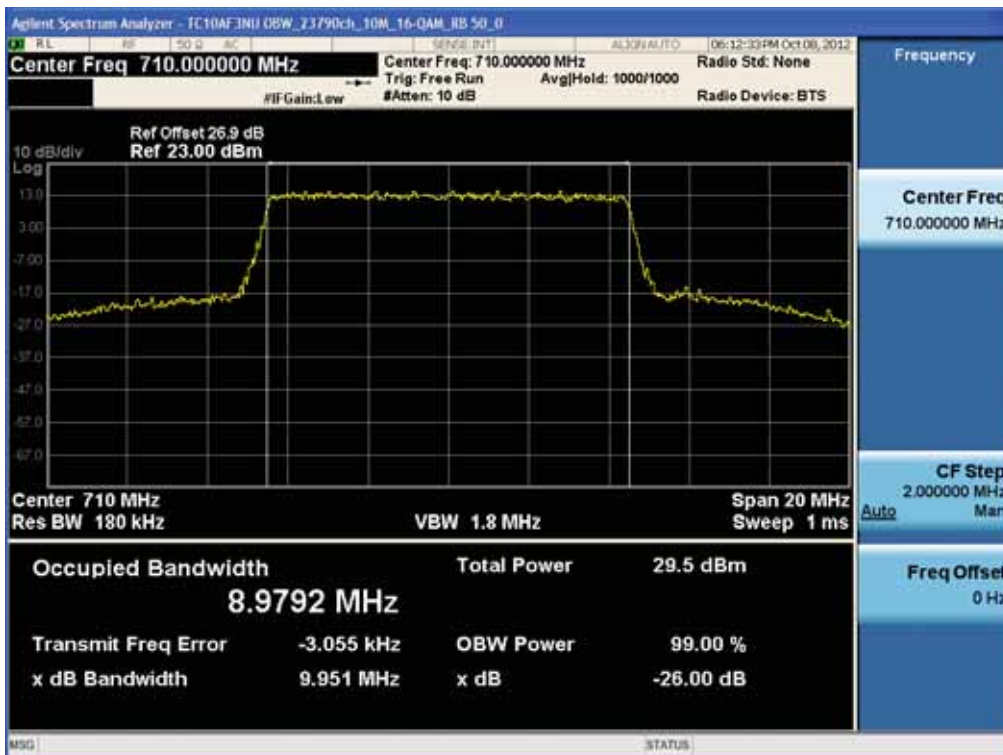
BAND 17. Occupied Bandwidth Plot (23790ch_10MHz_16-QAM_RB 50)
