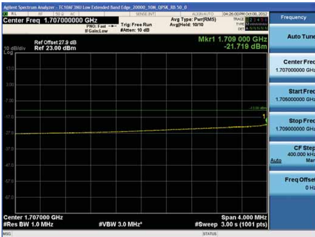
BAND 4. Low Extended Band Edge (20000ch_10MHz_QPSK_RB 50_0)
