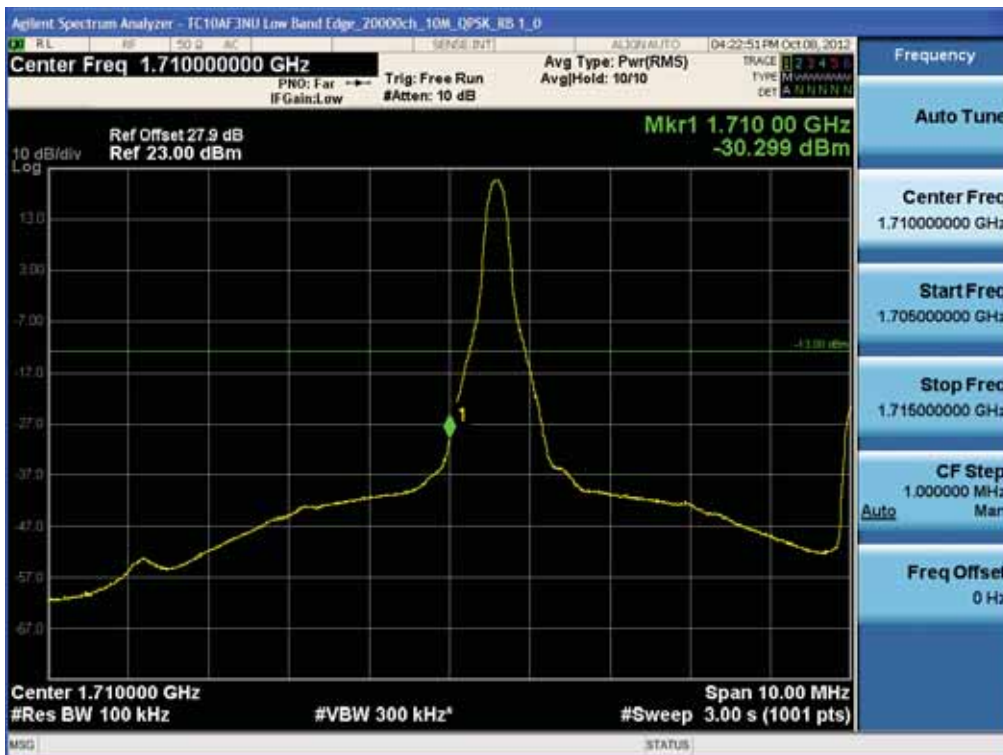
BAND 4. Low Band Edge Plot (20000ch_10MHz_QPSK_RB 1_0)
