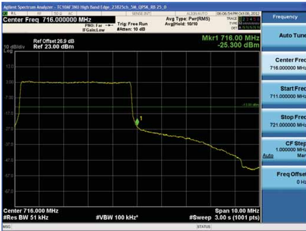
BAND 17. High Band Edge Plot (23825ch_5MHz_QPSK_RB 25_0)
