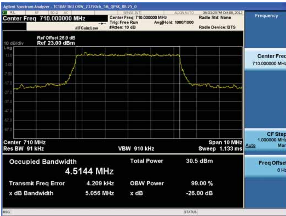
BAND 17. Occupied Bandwidth Plot (23790ch_5MHz_QPSK_RB 25)
