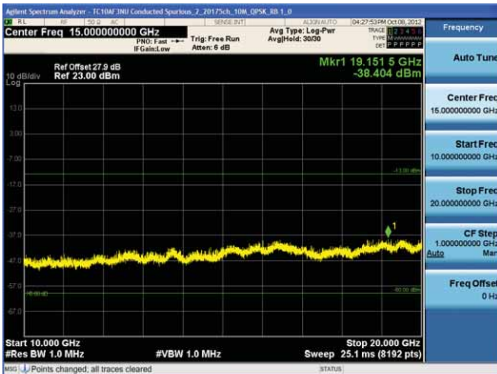
BAND 4. Conducted Spurious Plot_2 (20175ch_10MHz_QPSK_RB 1_0)
