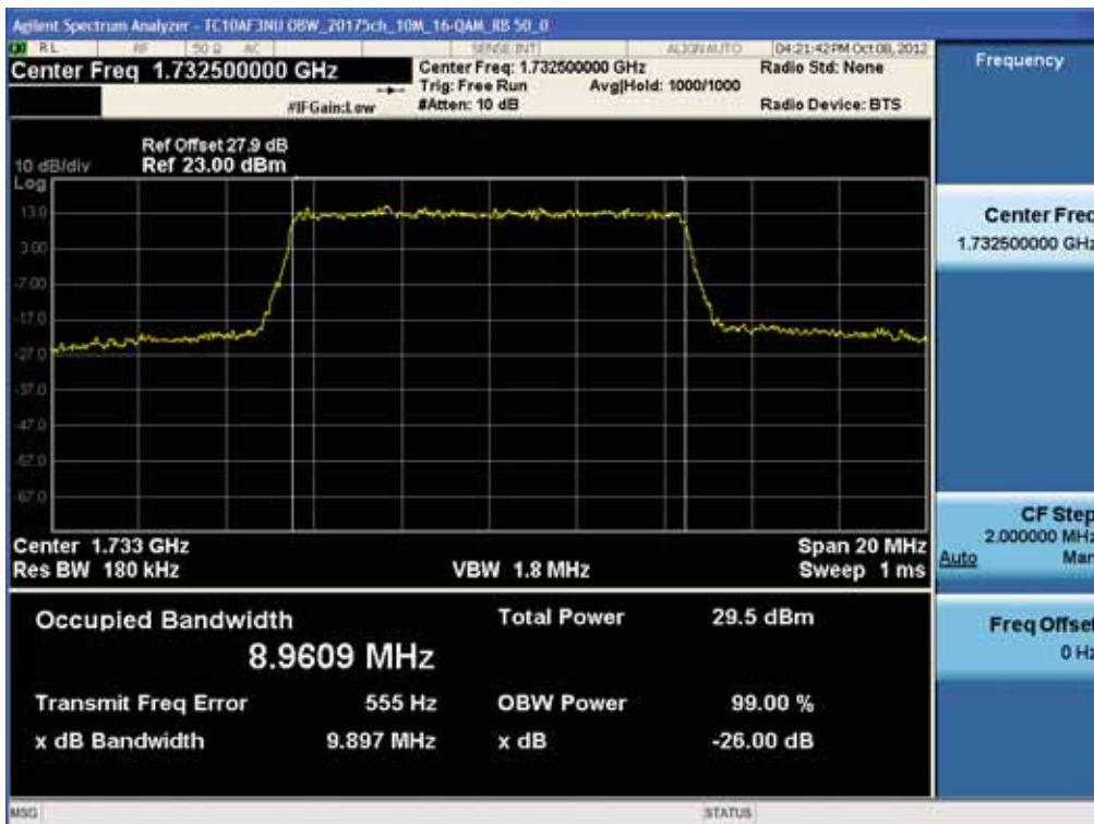
BAND 4. Occupied Bandwidth Plot (20175ch_10MHz_16-QAM_RB 50)
