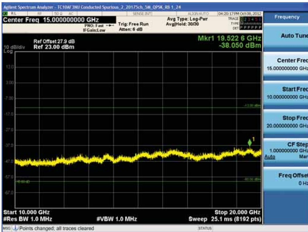
BAND 4. Conducted Spurious Plot_2 (20175ch_5MHz_QPSK_RB 1_24)
