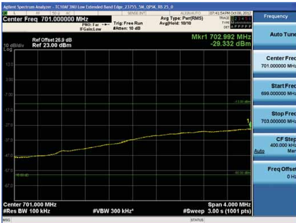
BAND 17. Low Extended Band Edge Plot (23755ch_5MHz_QPSK_RB 25_0)
