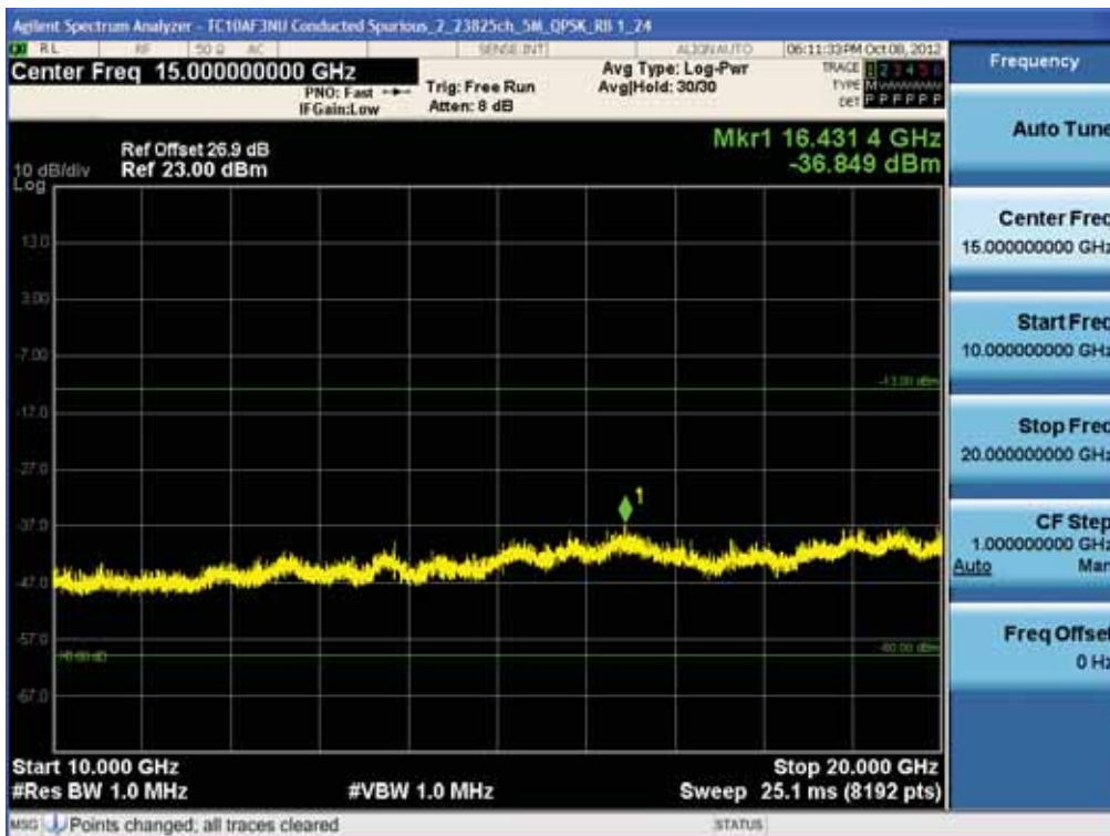
BAND 17. Conducted Spurious Plot_2 (23825ch_5MHz_QPSK_RB 1_24)
