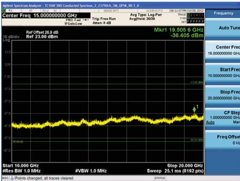
BAND 17. Conducted Spurious Plot_2 (23790ch_5MHz_QPSK_RB 1_0)
