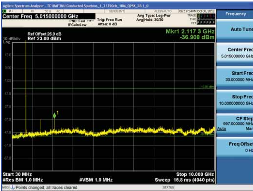
BAND 17. Conducted Spurious Plot_1 (23790ch_10MHz_QPSK_RB 1_0)
