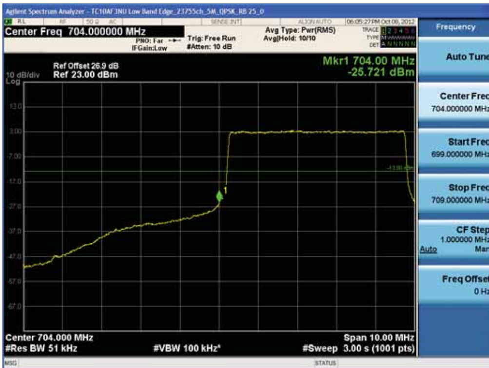
BAND 17. Low Band Edge Plot (23755ch_5MHz_QPSK_RB 25_0)
