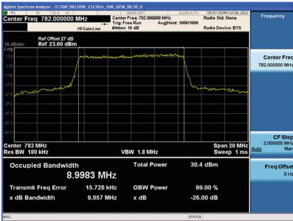
BAND 13. Occupied Bandwidth Plot (23230ch_10MHz_QPSK_RB 50)
