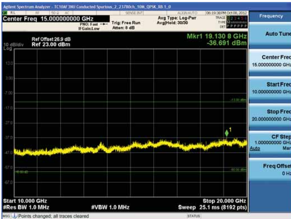
BAND 17. Conducted Spurious Plot_2 (23780ch_10MHz_QPSK_RB 1_0)
