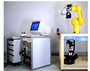
Fig. 1 SAR Test Setup
