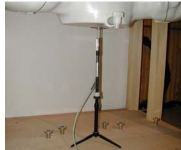
Figure 12.1 Dipole Validation Test Setup
