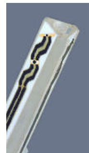
Figure 4.2 Probe Thick-Film Technique
