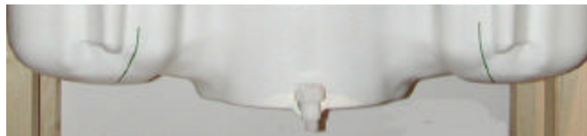
Figure 8.2 SAM Twin Phantom shell
