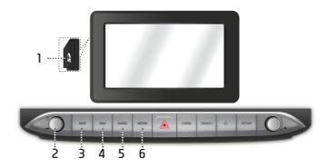
1. Cover for protecting SD card (SD card insert slot) Insert the SD card into the slot
