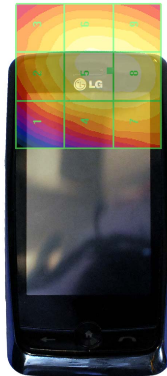
Figure 17-5 H-Field WD Scan overlay
