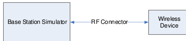
Figure 14-1 Power Measurement Setup
