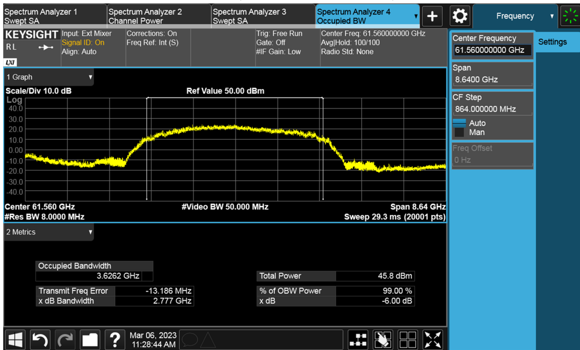
CH 10 Occupied Channel Bandwidth plot
