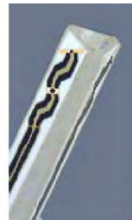
Figure E.2.2 Probe Thick-Film Technique
