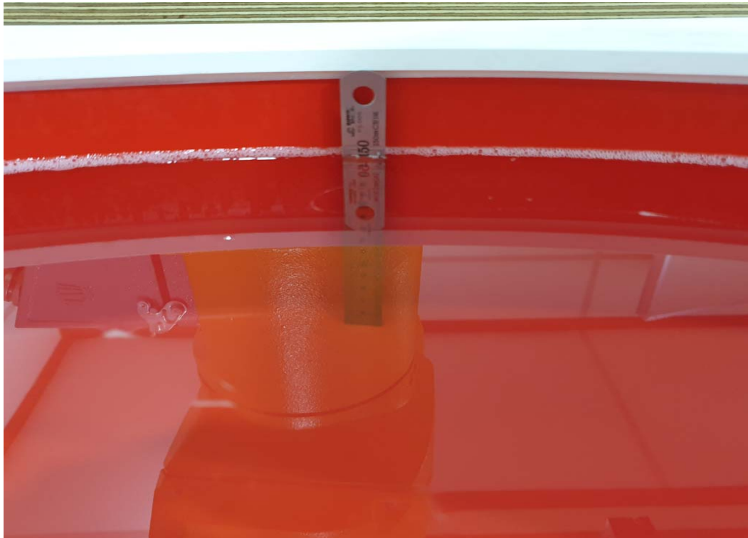
5 GHz (Head) Tissue Simulating Liquid, Depth: 150 mm
