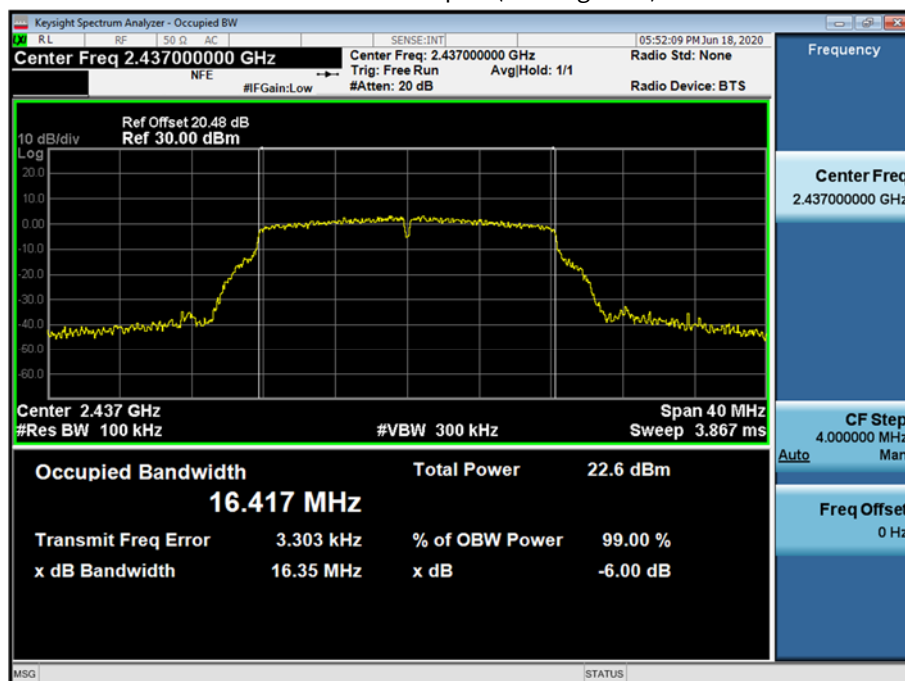
6dB Bandwidth plot (802.11g-CH 6)
