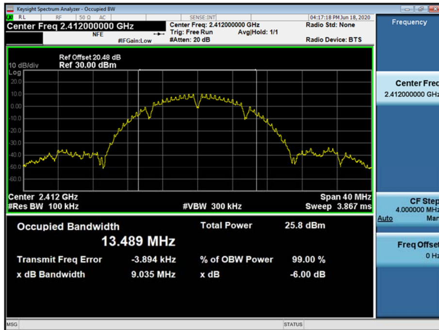
6dB Bandwidth plot (802.11b-CH 1)
