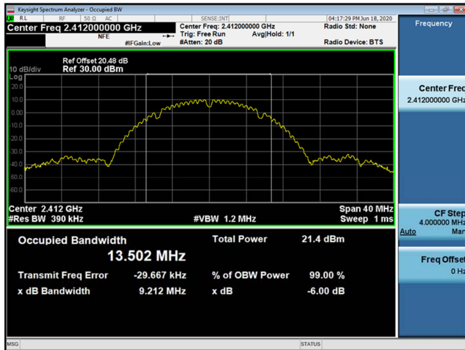
99% Bandwidth plot (802.11b-CH 1)
