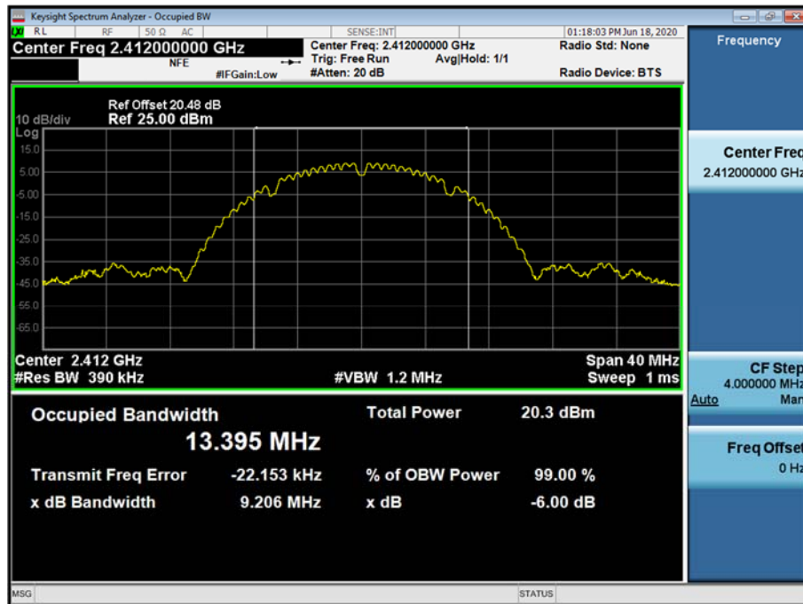
99% Bandwidth plot (802.11b-CH 1)
