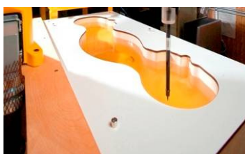
Figure 6-2 SAM Phantom with Simulating Tissue
