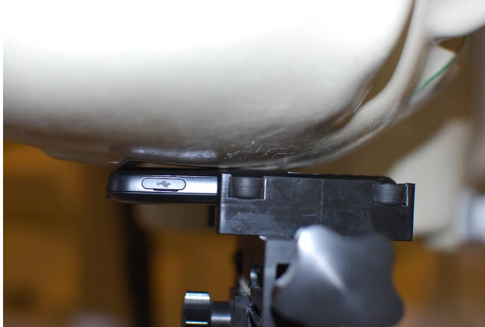
Figure 19-1 SAR Test Setup Photo 1
