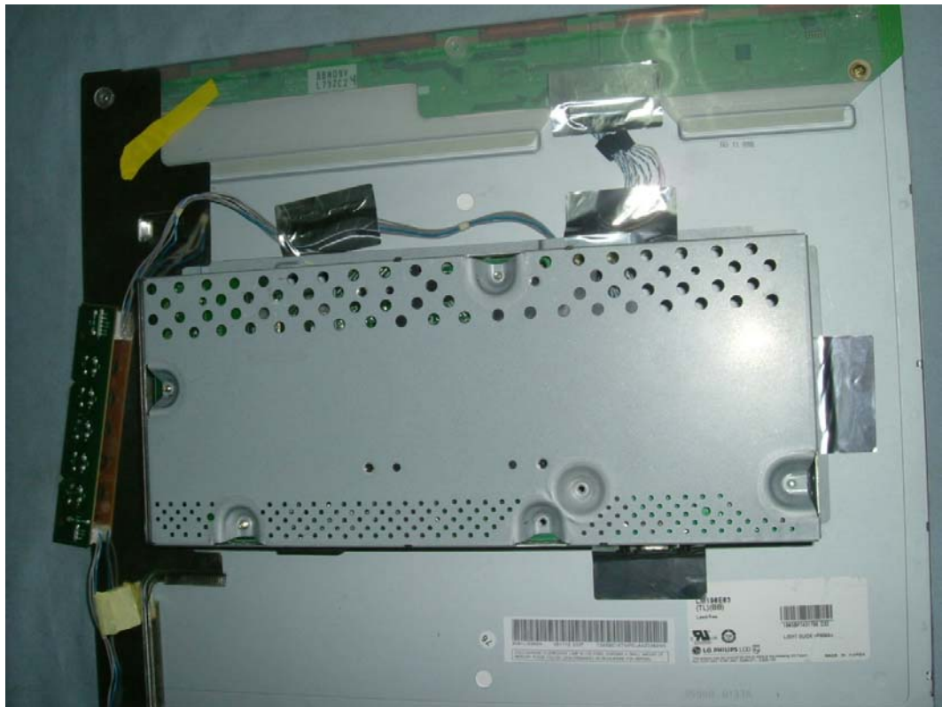
FIGURE 7 LCD MONITOR (M/N: L1952SQ) AL-TAPE
