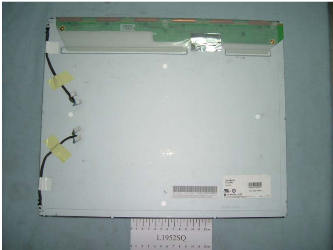
FIGURE 9 LCD MONITOR (M/N: L1952SQ) LCD PANEL
