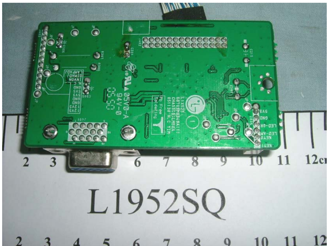
FIGURE 16 LCD MONITOR (M/N: L1952SQ) MAIN BOARD (SOLDERED SIDE)
