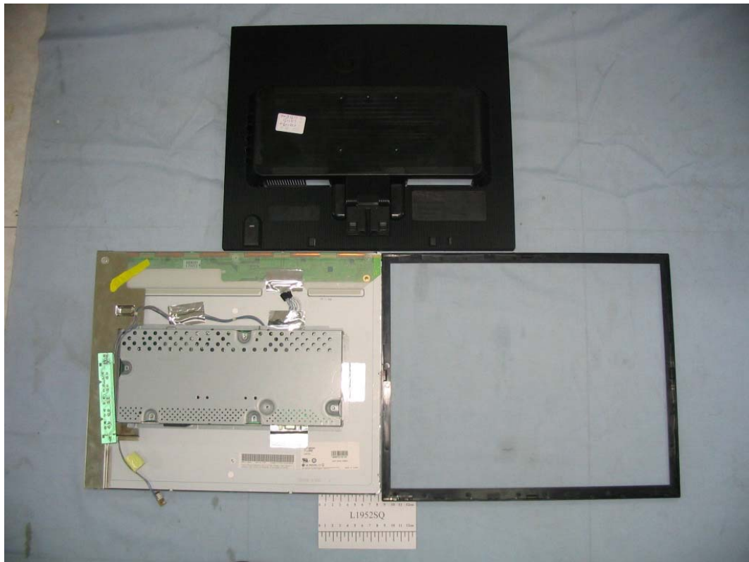
FIGURE 5 LCD MONITOR (M/N: L1952SQ) COVER REMOVED 1
