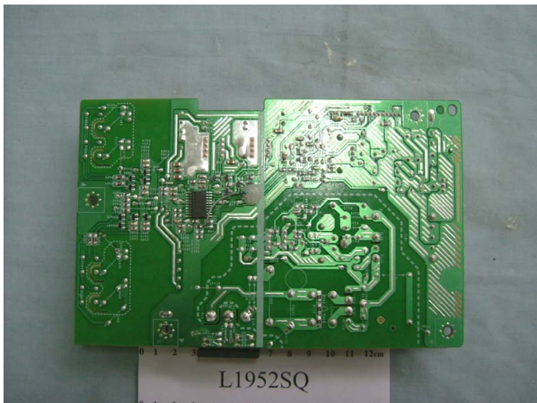
FIGURE 14 LCD MONITOR (M/N: L1952SQ) POWER BOARD (SOLDERED SIDE)
