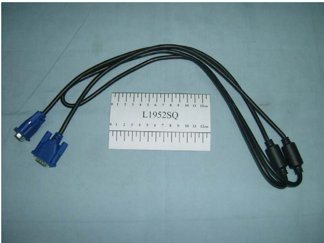
FIGURE 2 LCD MONITOR (M/N: L1952SQ) D-SUB CABLE
