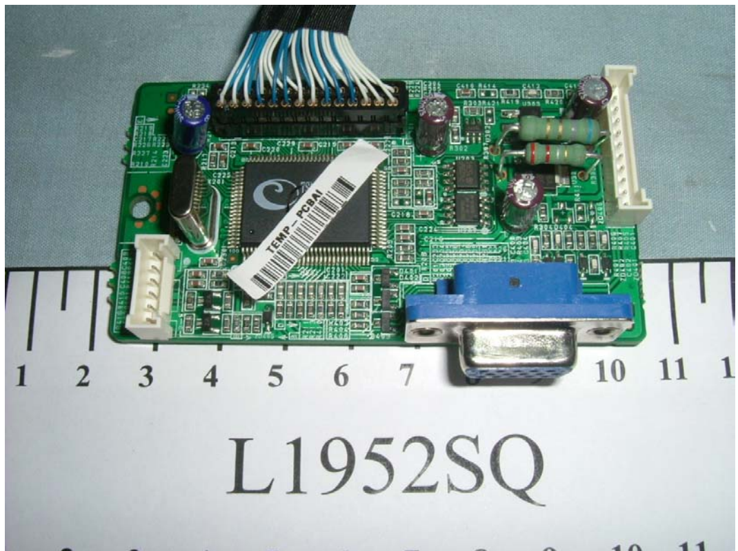
FIGURE 15 LCD MONITOR (M/N: L1952SQ) MAIN BOARD (COMPONENT SIDE)
