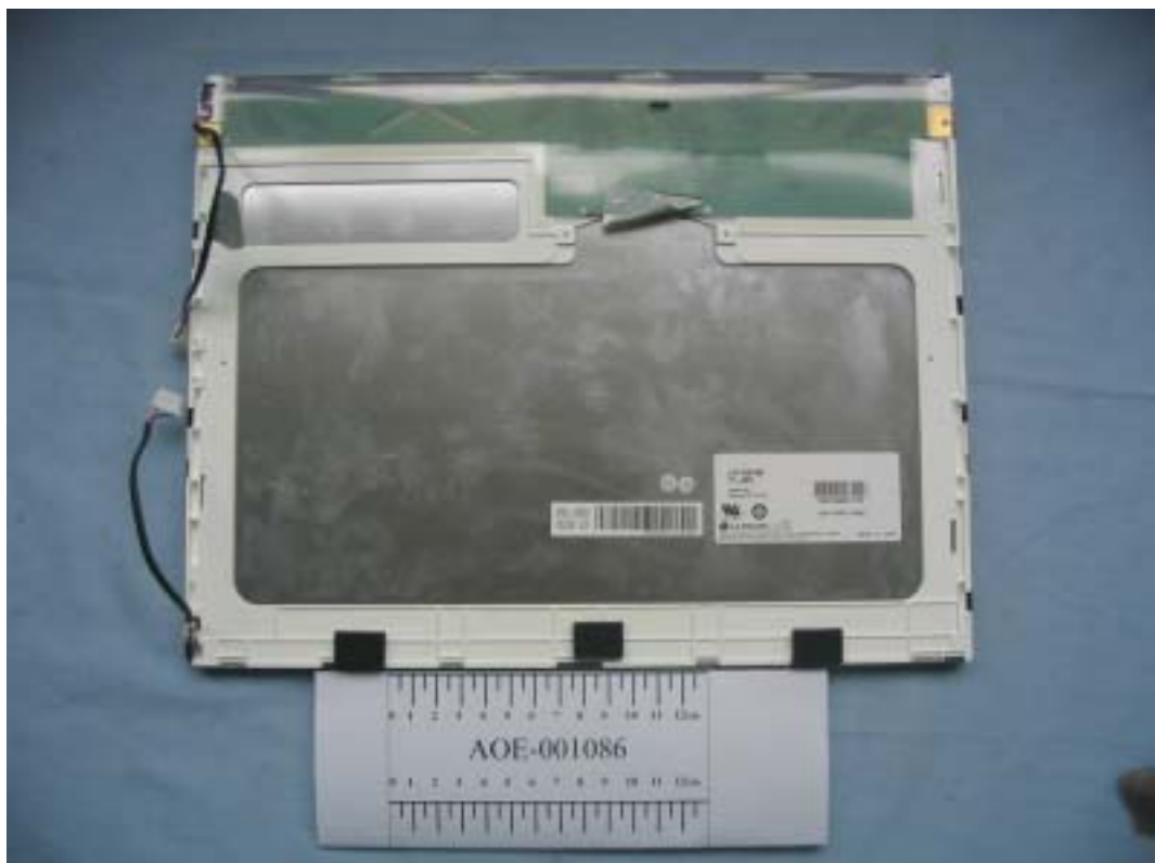
FIGURE 4 LCD MONITOR (M/N: L1552SQ) LCD PANEL (REAR VIEW)
