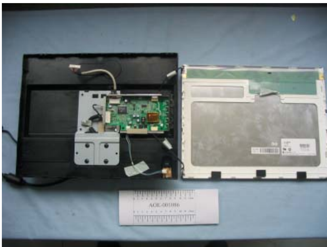
FIGURE 2 LCD MONITOR (M/N: L1552SQ) REAR COVER REMOVED
