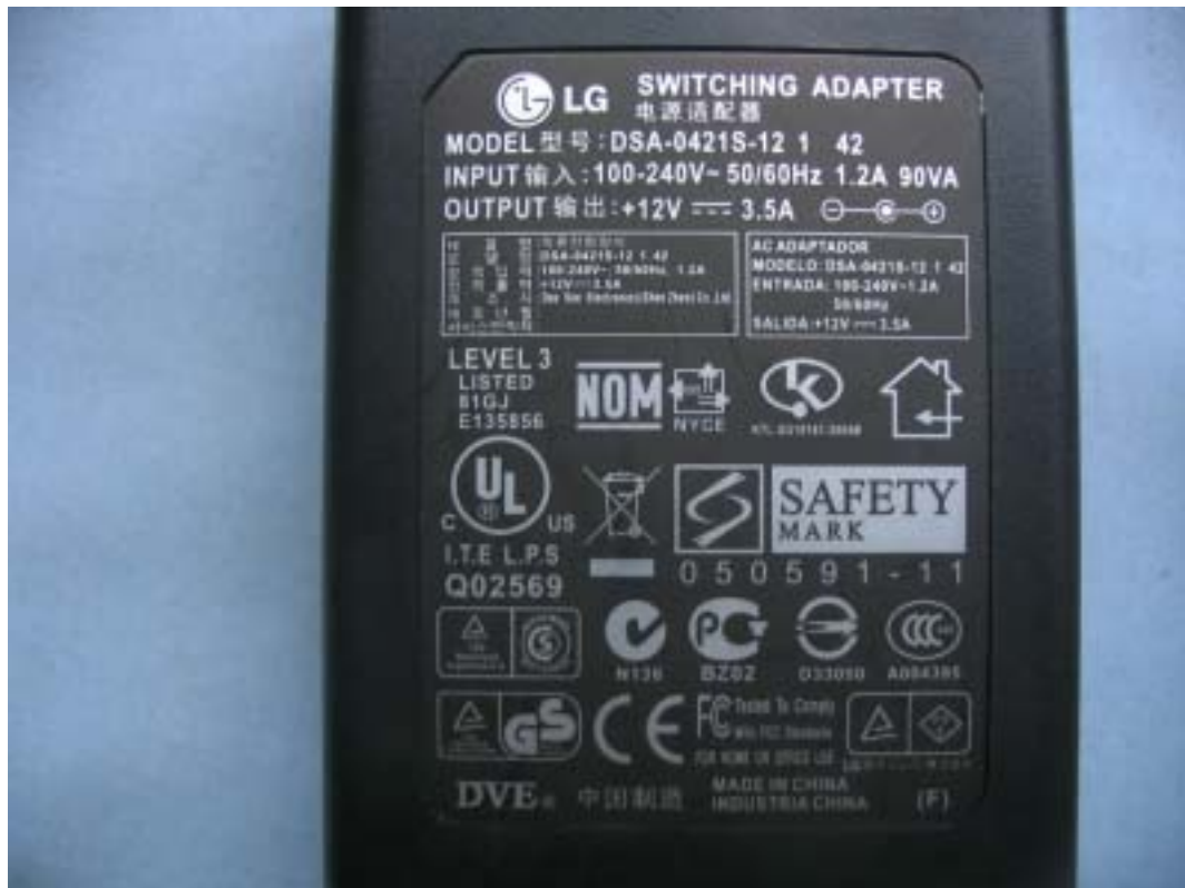
FIGURE 13 LCD MONITOR (M/N: L1552SQ) ADAPTOR - LABEL
