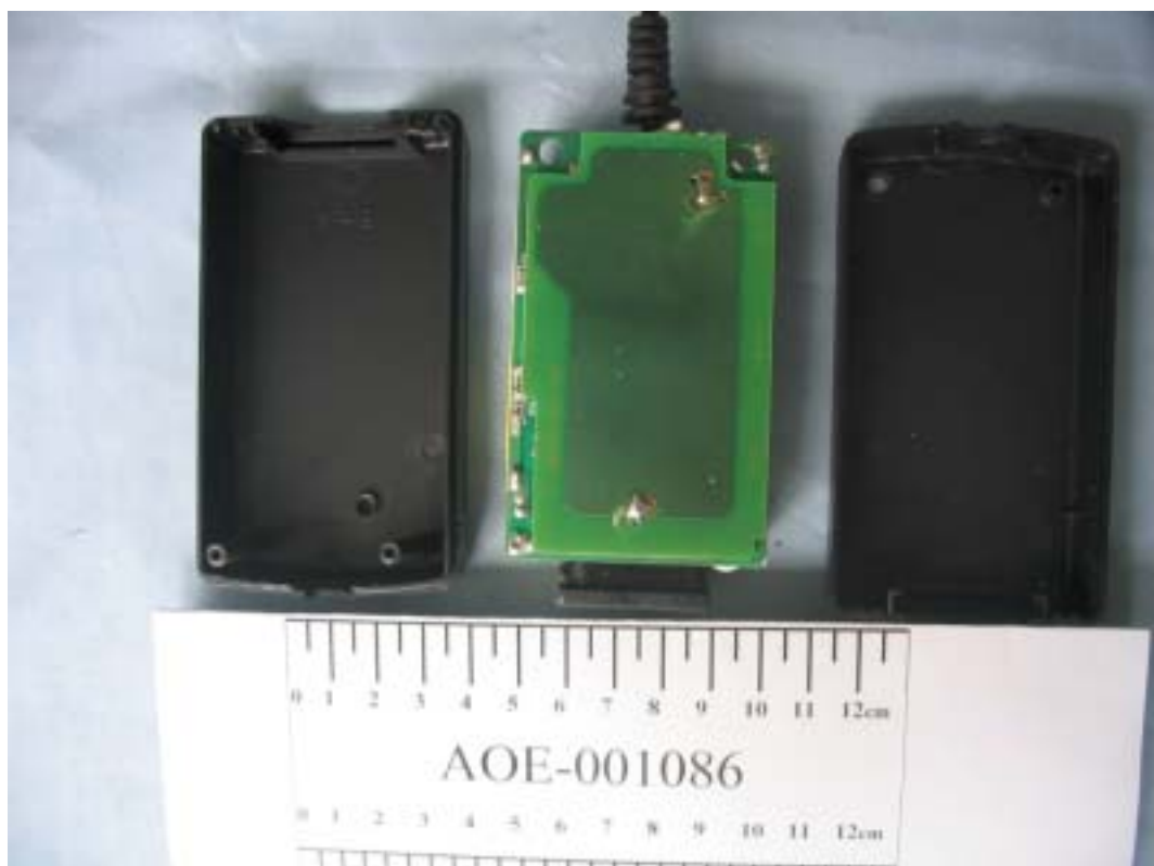
FIGURE 14 LCD MONITOR (M/N: L1552SQ) ADAPTOR - COVER REMOVED
