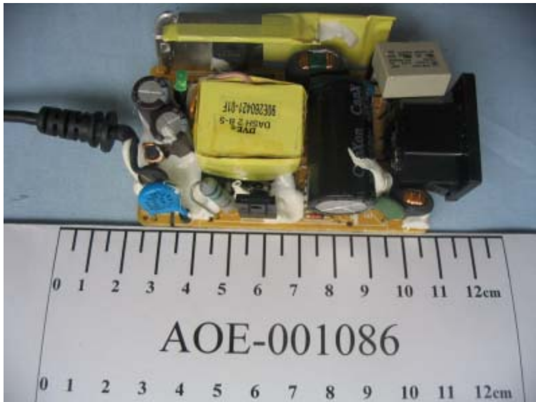
FIGURE 16 LCD MONITOR (M/N: L1552SQ) ADAPTOR – COMPONENT SIDE
