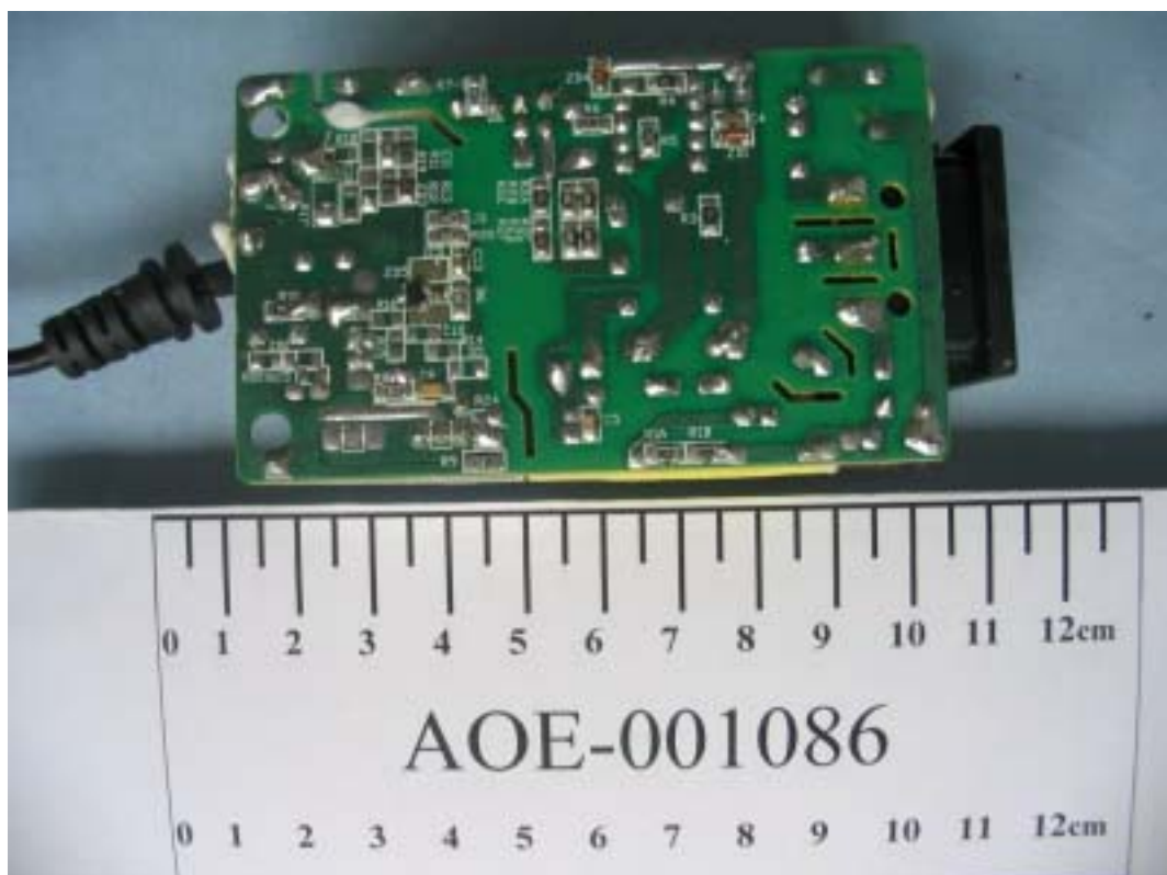
FIGURE 17 LCD MONITOR (M/N: L1552SQ) ADAPTOR – SOLDERED SIDE
