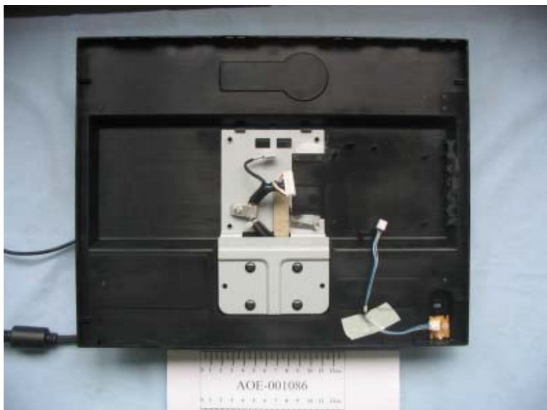
FIGURE 6 LCD MONITOR (M/N: L1552SQ) MAIN BOARD REMOVED
