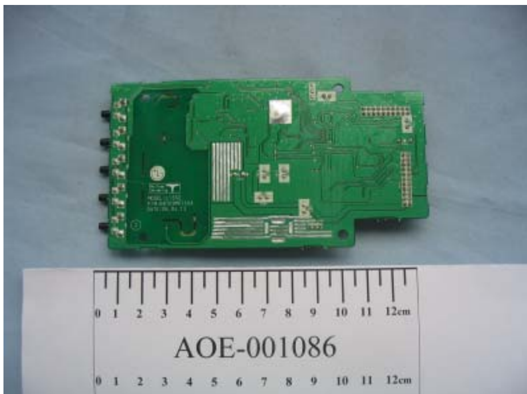
FIGURE 9 LCD MONITOR (M/N: L1552SQ) MAIN BOARD (SOLDERED SIDE)
