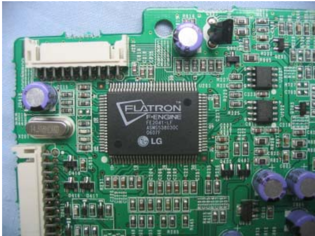
FIGURE 10 LCD MONITOR (M/N: L1552SQ) MAIN BOARD - IC
