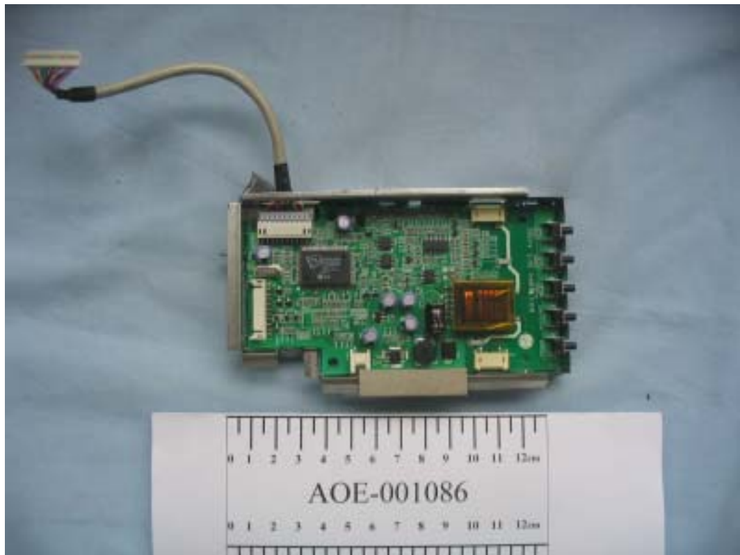
FIGURE 7 LCD MONITOR (M/N: L1552SQ) MAIN BOARD WITH MENTAL CASE
