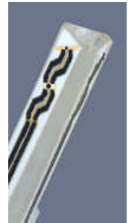
Figure 3.2 Probe Thick-Film Technique
