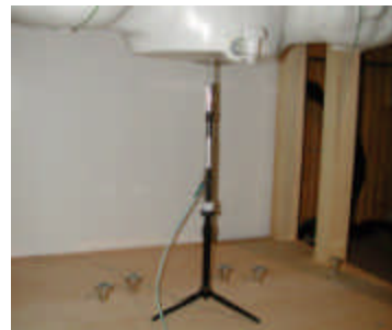
Figure 12.1 Dipole Validation Test Setup
