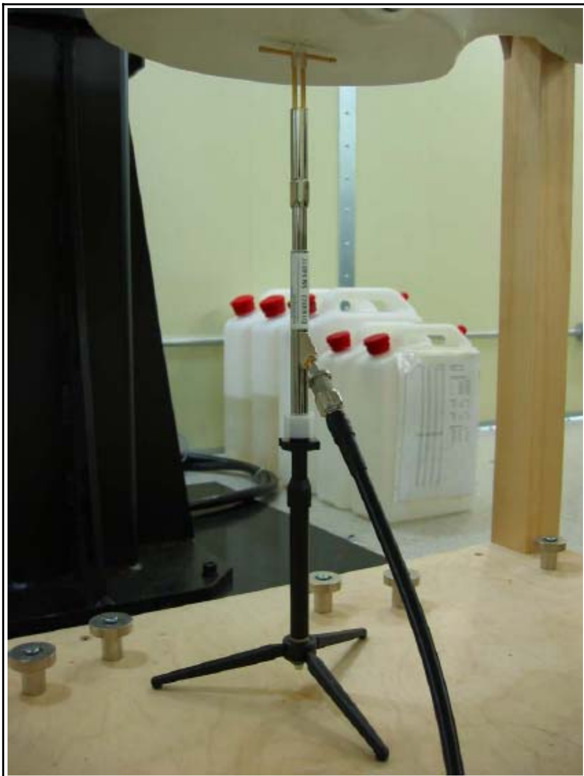
Figure 1 1900 MHz Dipole Validation Test Setup
