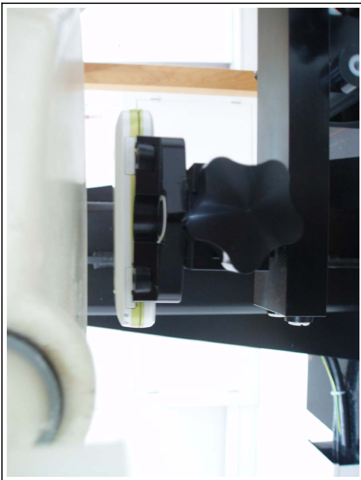
Figure 6 Body SAR Test Setup – w/o Holster
