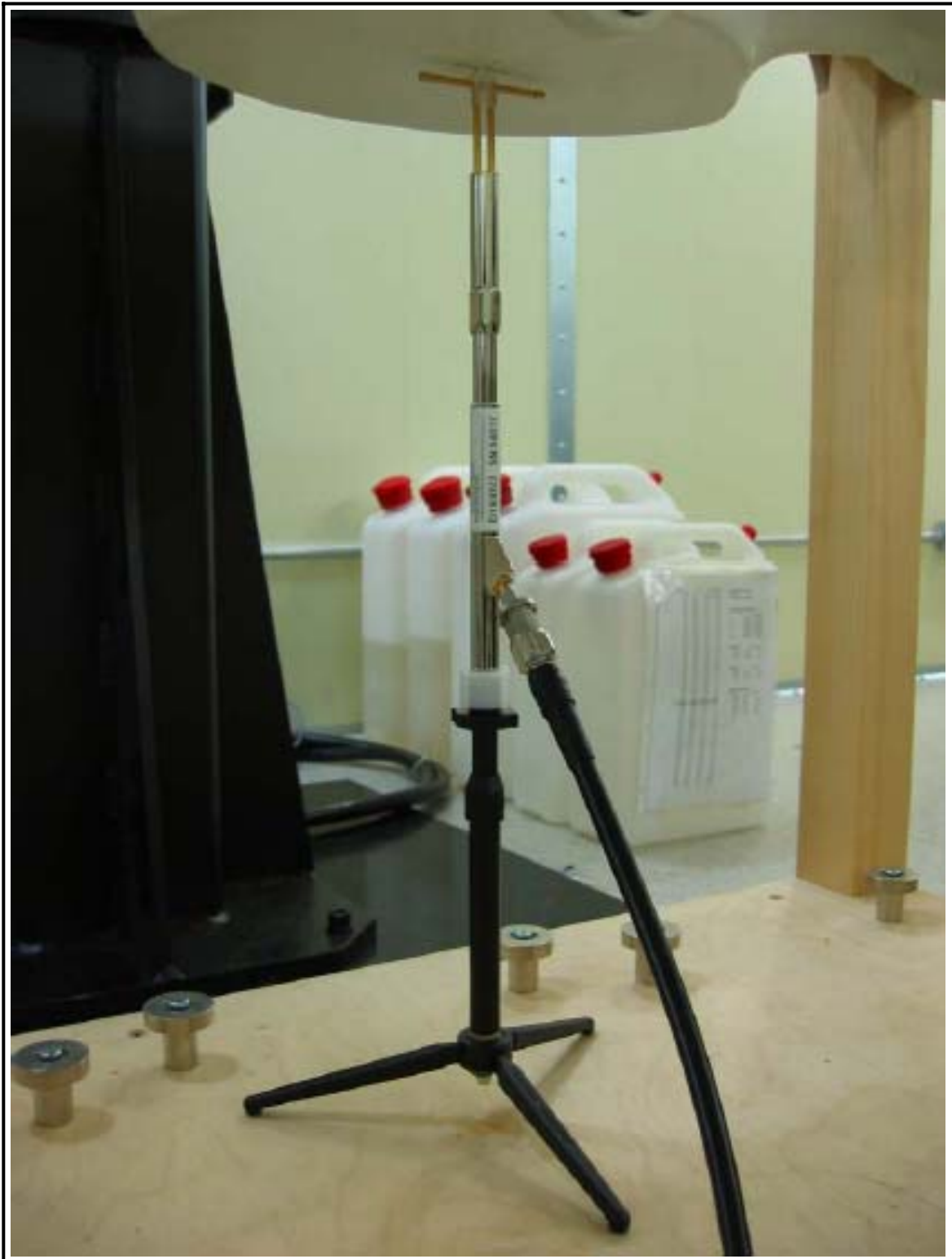
Figure 1 1900 MHz Dipole Validation Test Setup
