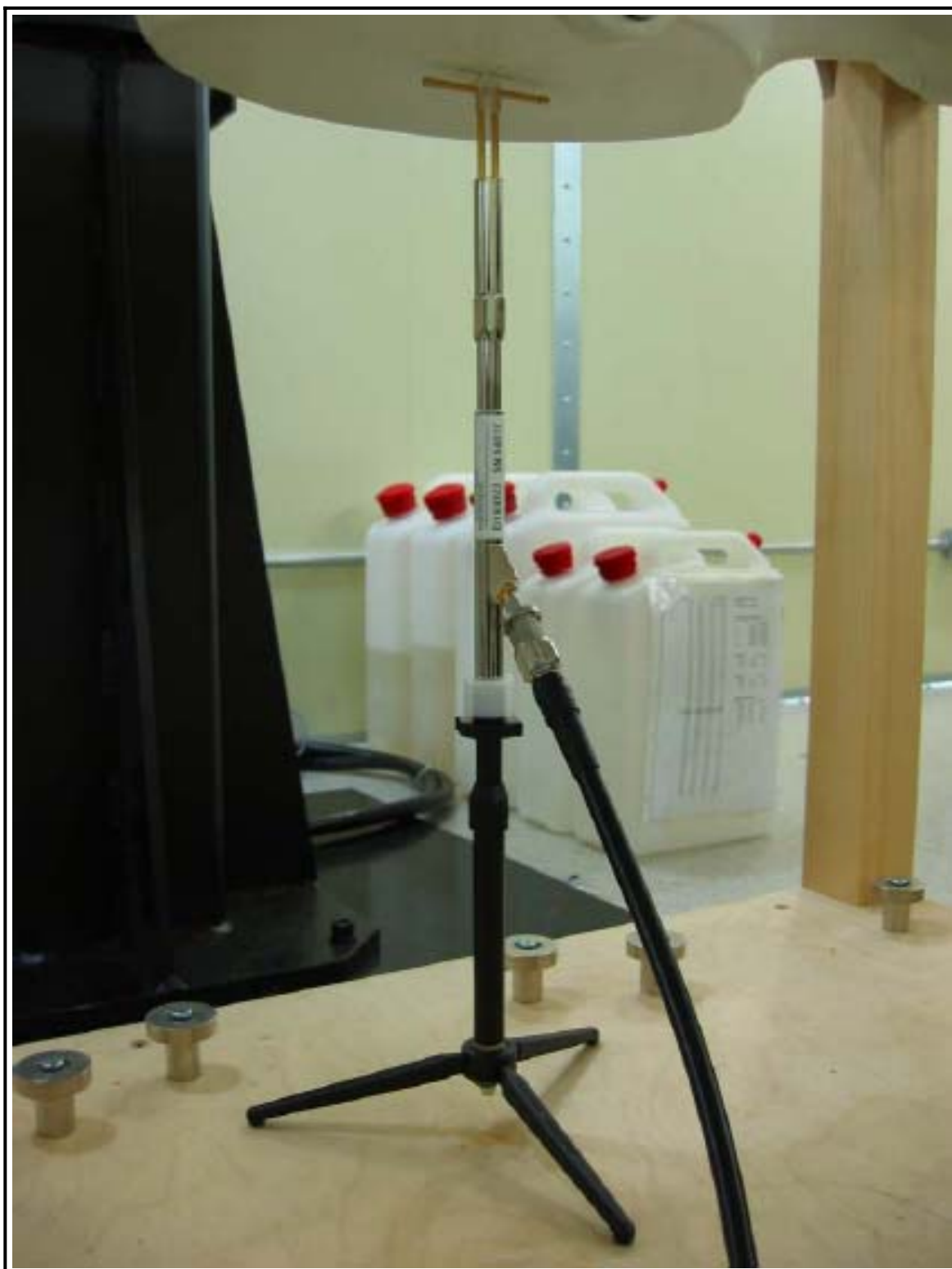
Figure 1 1900 MHz Dipole Validation Test Setup
