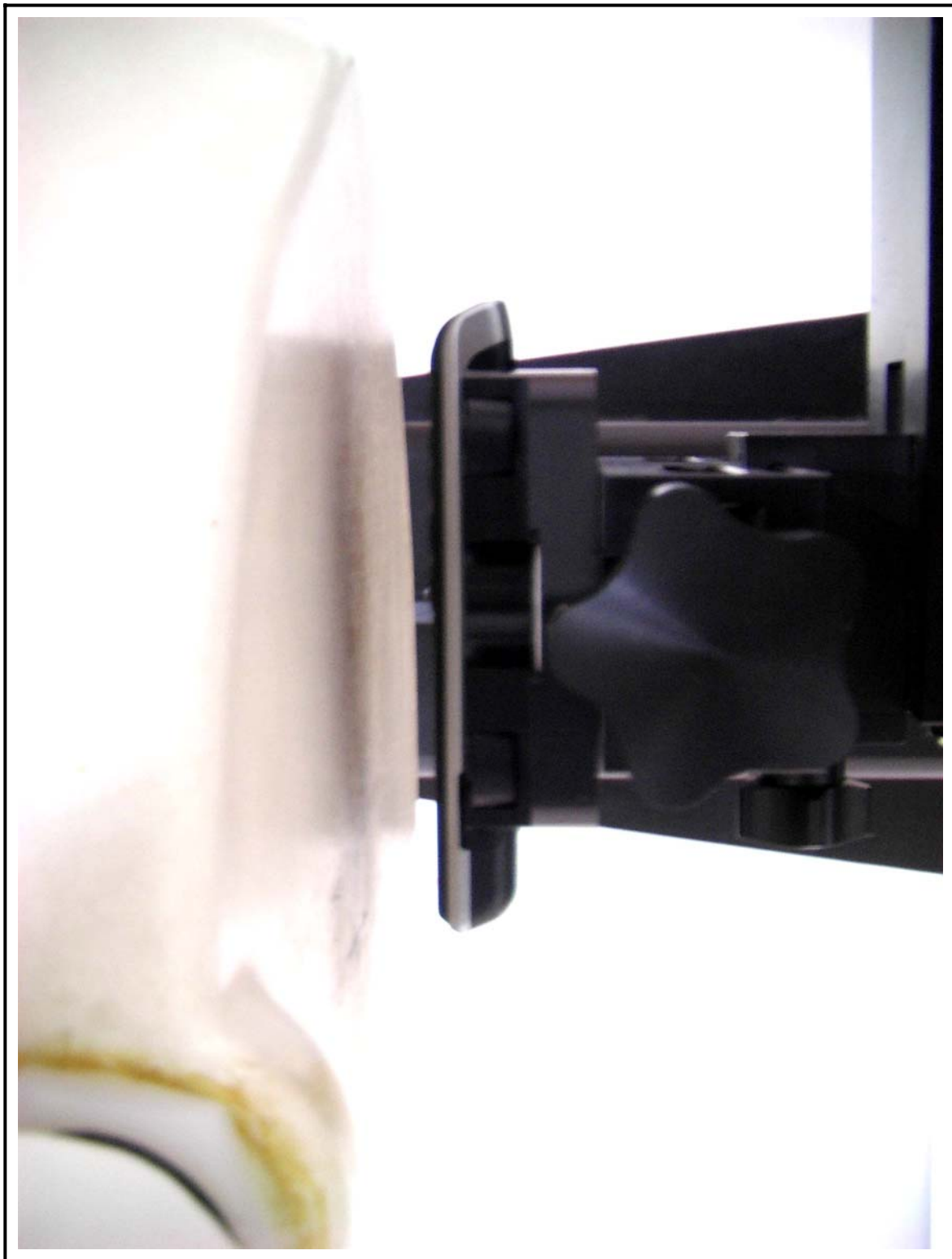
Figure 6 Body SAR Test Setup – w/o Holster
