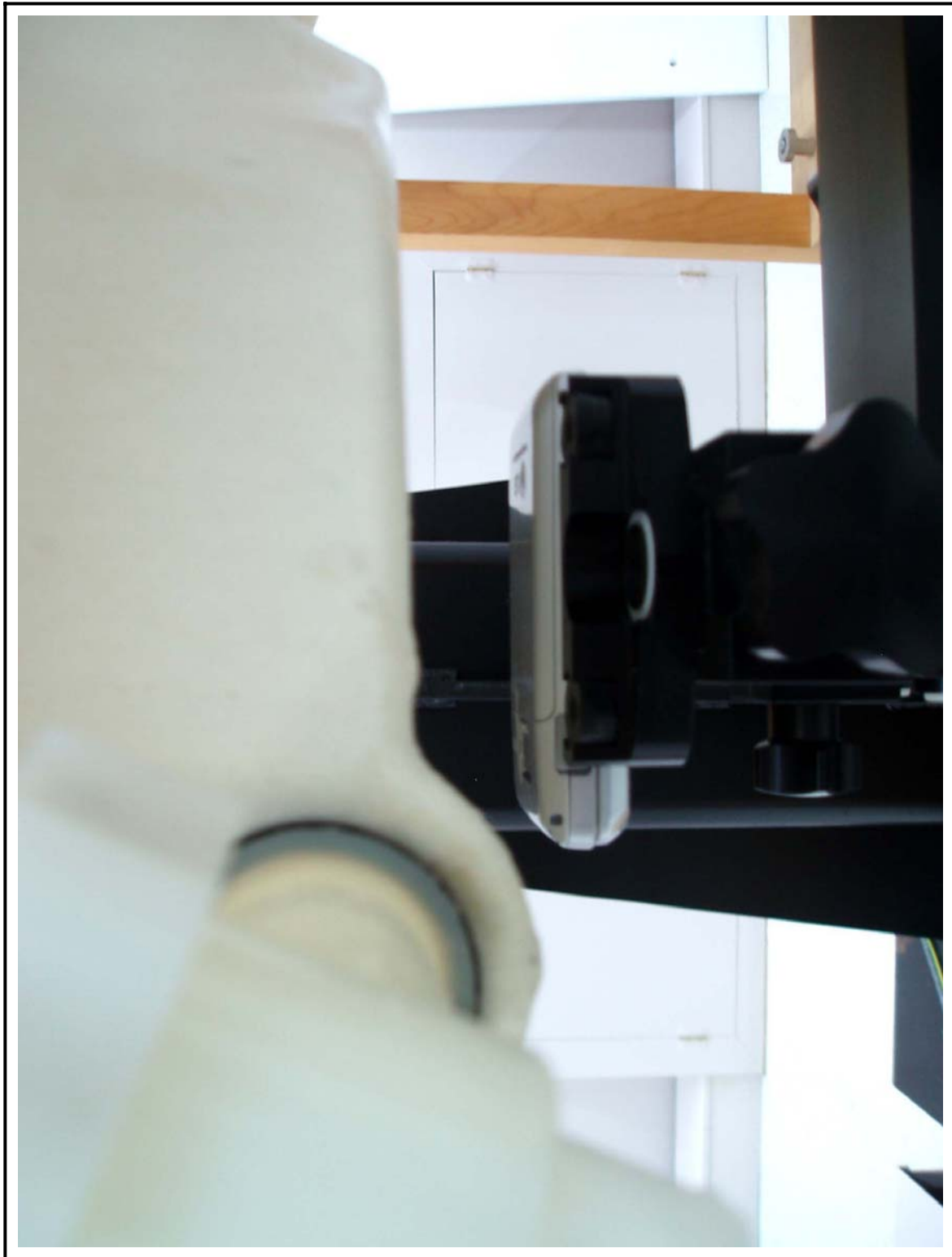
Figure 27 Body SAR Test Setup – w/o Holster
