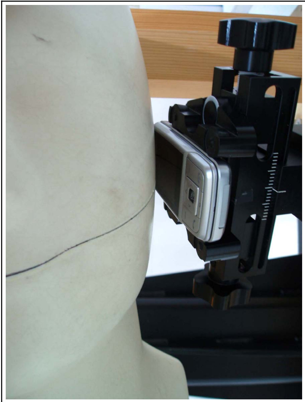
Figure 20 Left Head SAR Test Setup – Ear Tilt Position
