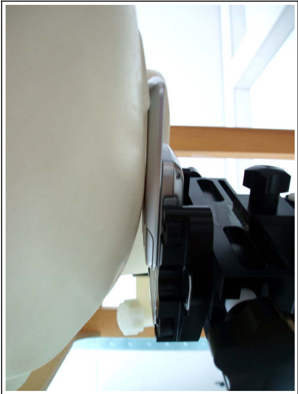
Figure 18 Left Head SAR Test Setup – Cheek Touch Position
