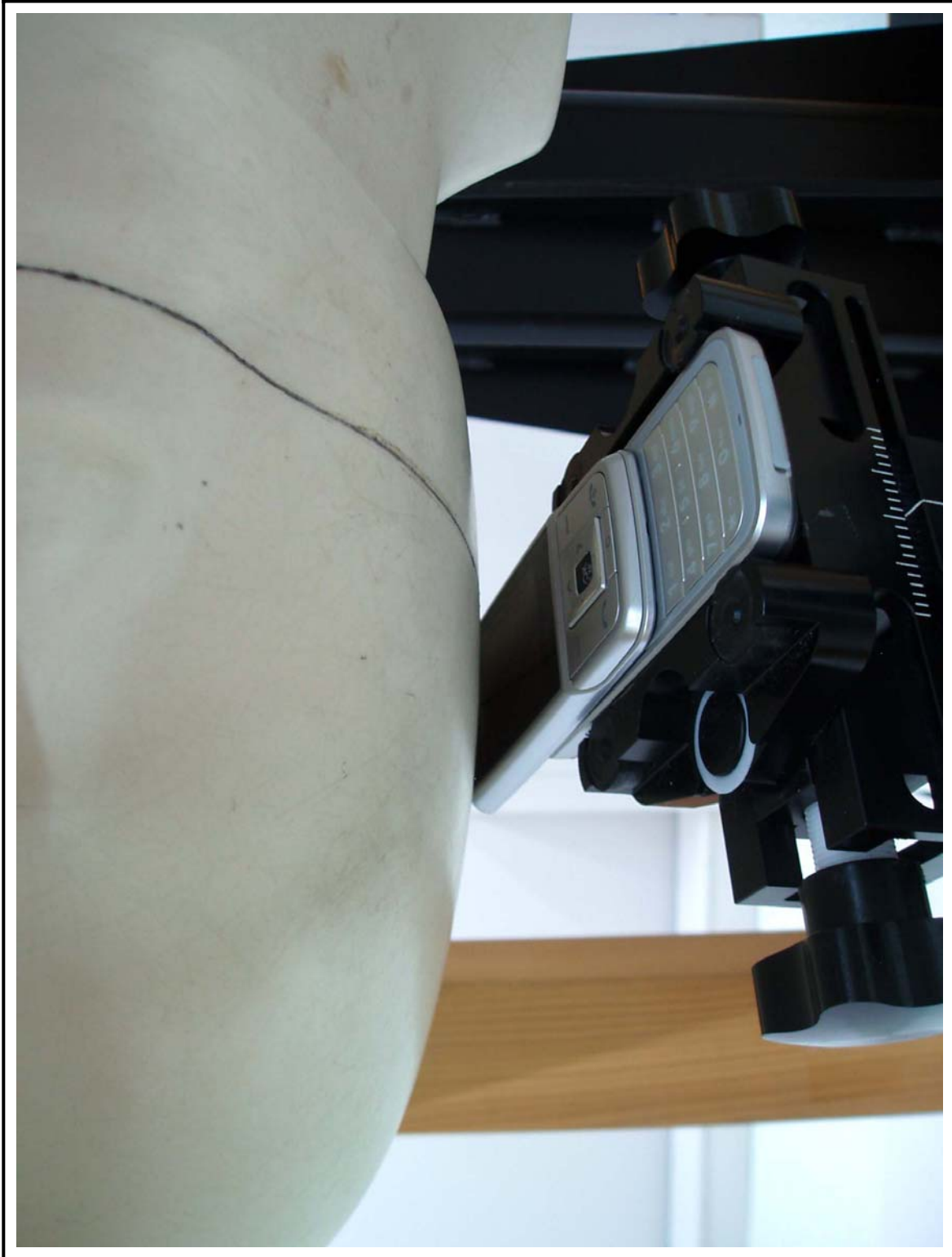
Figure 11 Right Head SAR Test Setup - Ear Tilt Position
