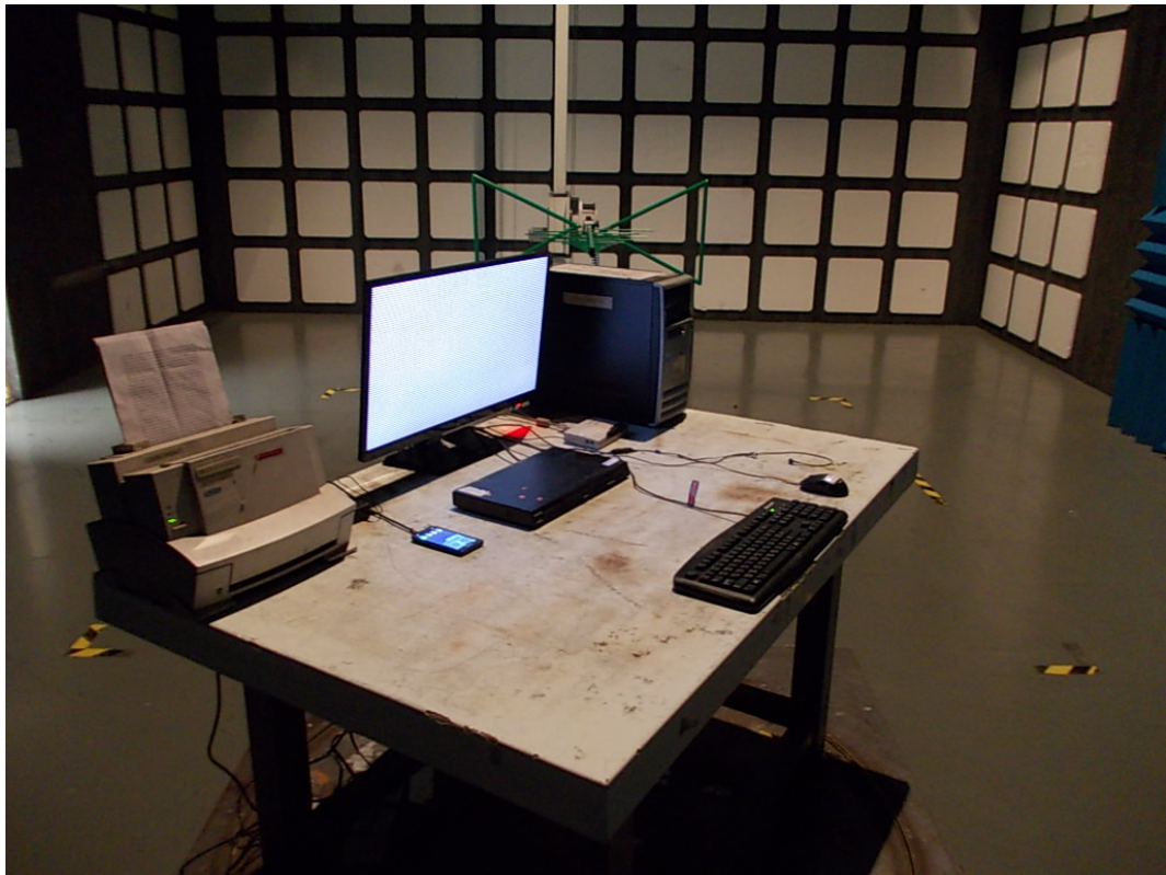
SETUP WITH MAXIMUM DETECTED EMISSION AT HORIZONTAL POLARIZATION (TEST MODE: HDMI 1920*1080@60Hz ADAPTER #3)
