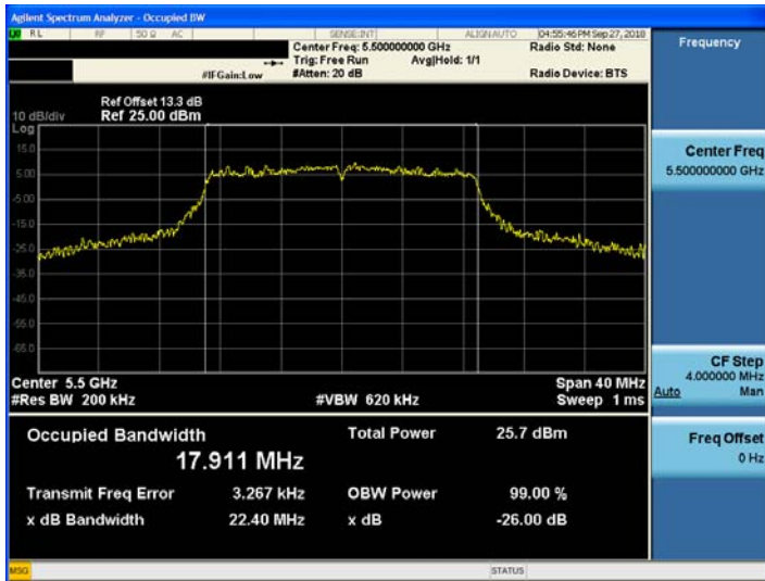
802.11n_HT20 UNII 2C BAND 26dB Bandwidth(CH 100)
