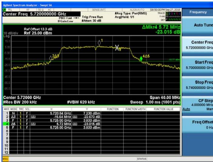
802.11ac_VHT20 CH.144 Bandwidth
