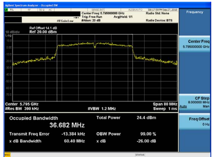
802.11ac_VHT40 UNII 3 BAND 26dB Bandwidth (CH 159)
