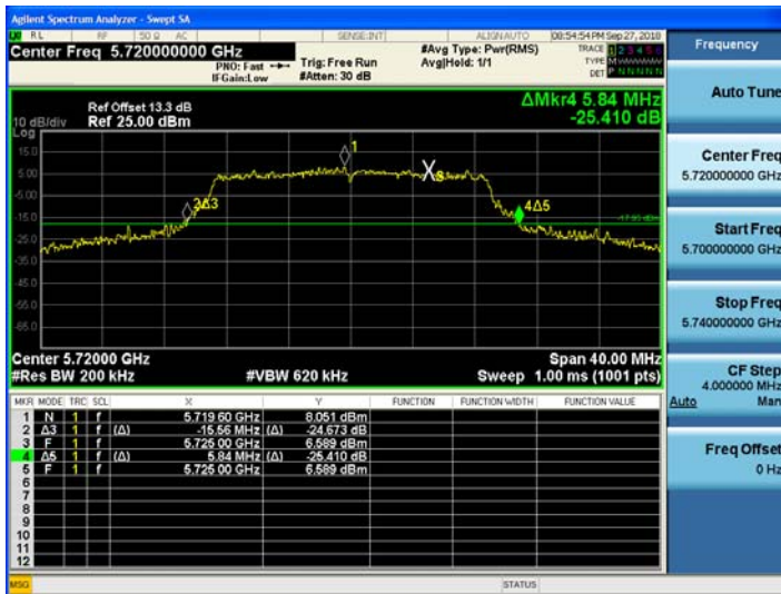
802.11ac_VHT20 CH.144 Bandwidth
