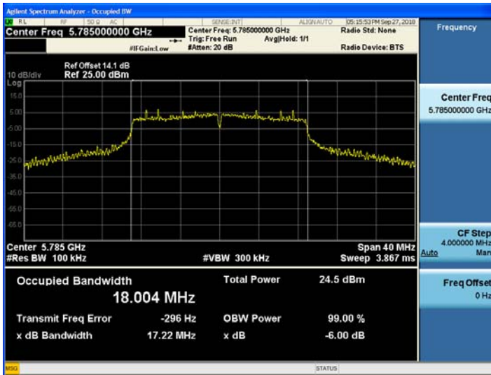
802.11ac_VHT20 UNII 3 BAND 6dB Bandwidth(CH.157)
