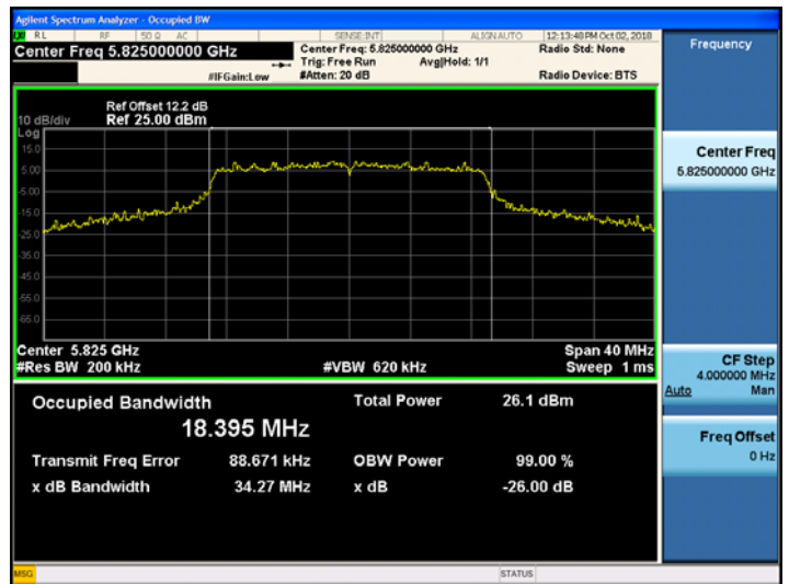
802.11n_HT20 UNII 3 BAND 26dB Bandwidth(CH 165)
