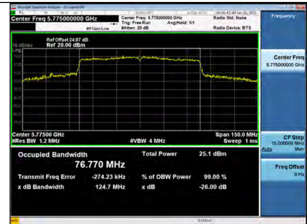
802.11ac_VHT80 UNII 3 BAND 26dB Bandwidth (CH 155)
