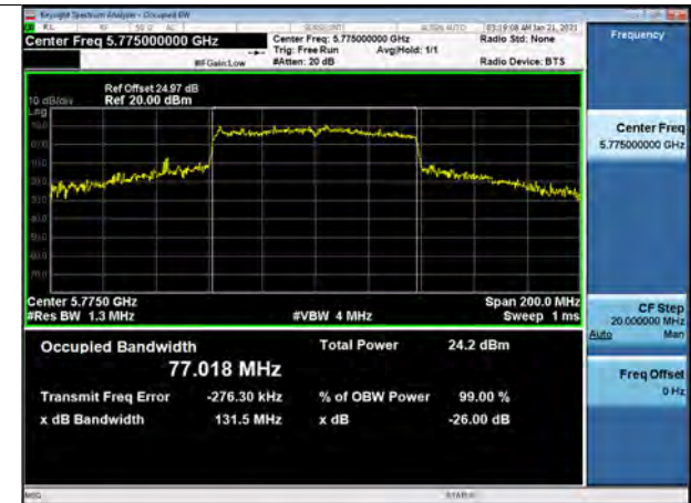
802.11ac_VHT80 UNII 3 BAND 26dB Bandwidth (CH 155)
