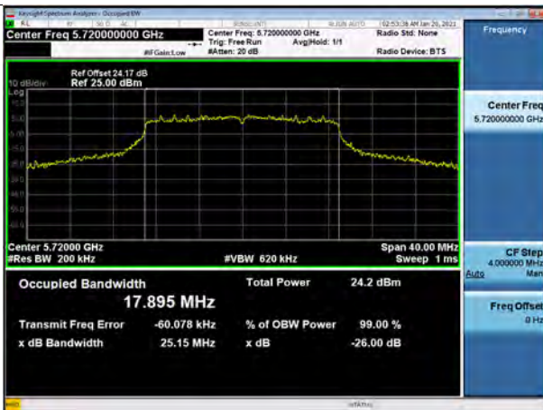
802.11n_HT20 UNII 2C BAND 26dB Bandwidth(CH 144)
