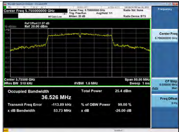
802.11ac_VHT40 UNII 3 BAND 26dB Bandwidth (CH 151)
