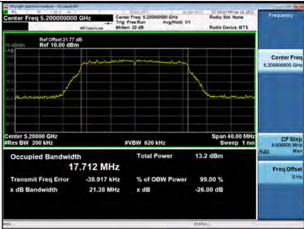
802.11ac_VHT20 UNII 2C BAND 26dB Bandwidth(CH 144)
