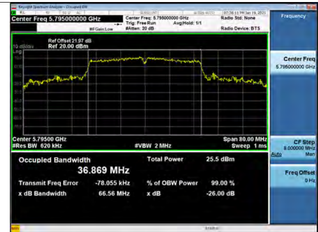
802.11ac_VHT40 UNII 3 BAND 26dB Bandwidth (CH 159)
