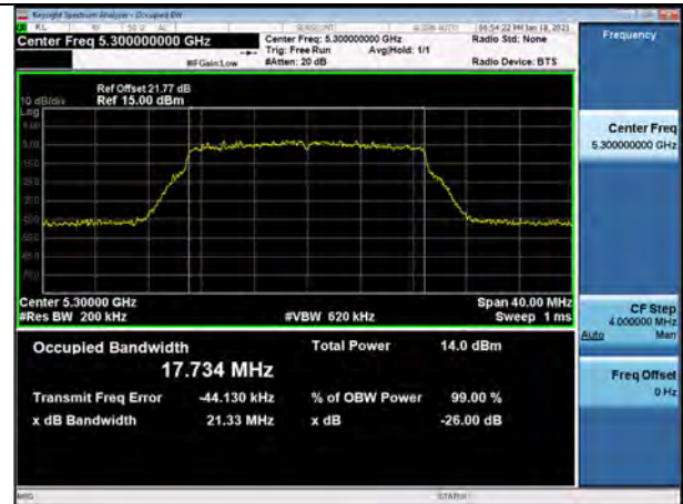
802.11n_HT20 UNII 3 BAND 26dB Bandwidth(CH 149)
