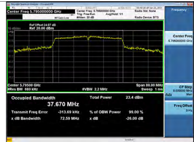
802.11ac_VHT40 UNII 3 BAND 26dB Bandwidth (CH 159)
