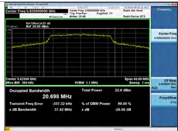
802.11n_HT20 UNII 3 BAND 26dB Bandwidth(CH 165)
