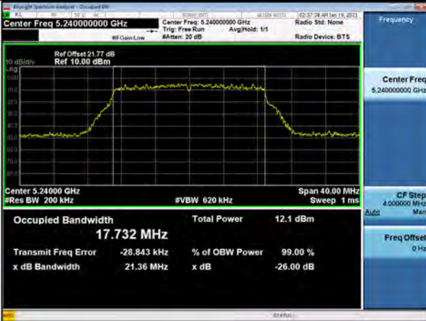
802.11n_HT20 UNII 2C BAND 26dB Bandwidth(CH 144)
