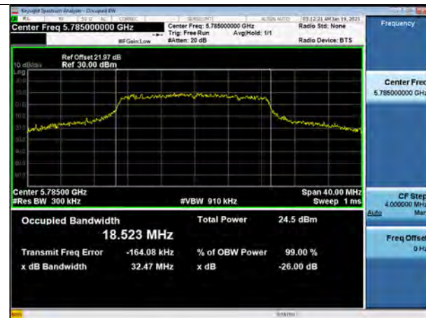
802.11ac_VHT20 UNII 3 BAND 26dB Bandwidth(CH 157)
