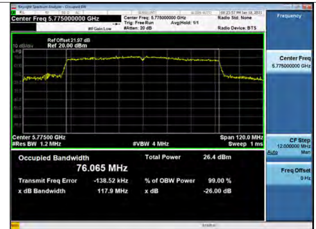
802.11ac_VHT80 UNII 3 BAND 26dB Bandwidth (CH 155)
