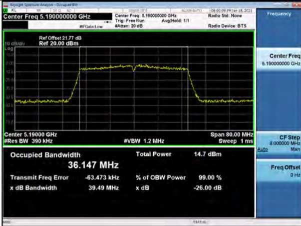
802.11ac_VHT40 UNII 2C BAND 26dB Bandwidth(CH 142)
