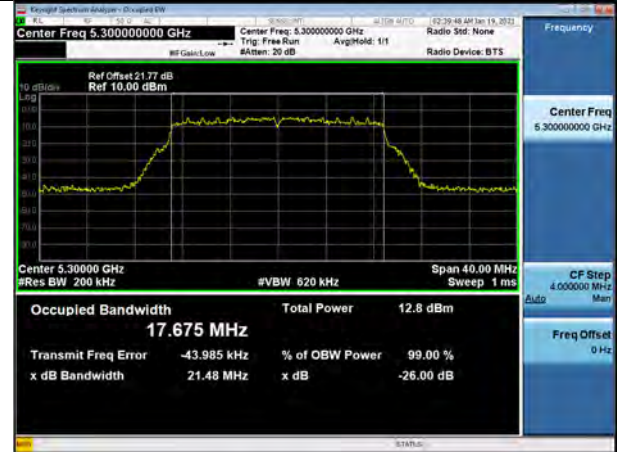
802.11n_HT20 UNII 3 BAND 26dB Bandwidth(CH 157)
