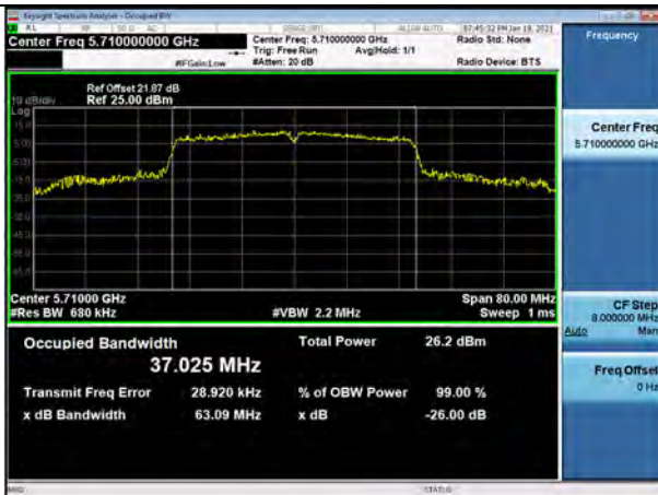
802.11n_HT40 UNII 2C BAND 26dB Bandwidth(CH 142)
