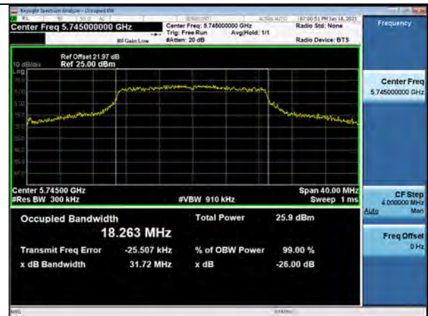
802.11n_HT20 UNII 3 BAND 26dB Bandwidth(CH 149)
