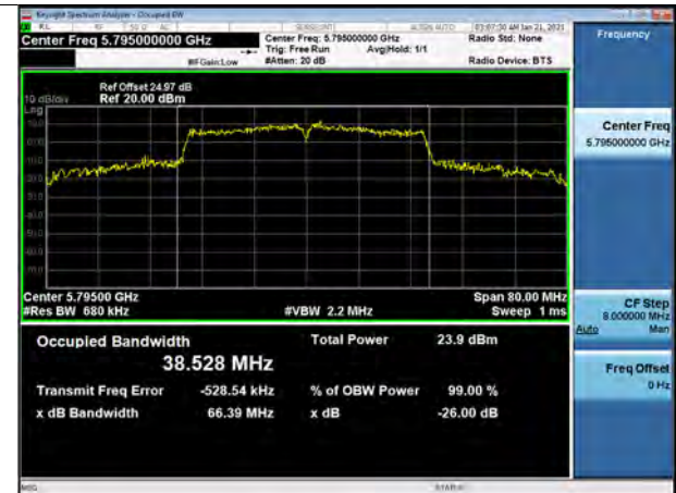
802.11ac_VHT40 UNII 3 BAND 26dB Bandwidth (CH 159)
