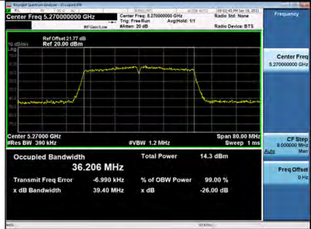
802.11ac_VHT40 UNII 3 BAND 26dB Bandwidth (CH 151)
