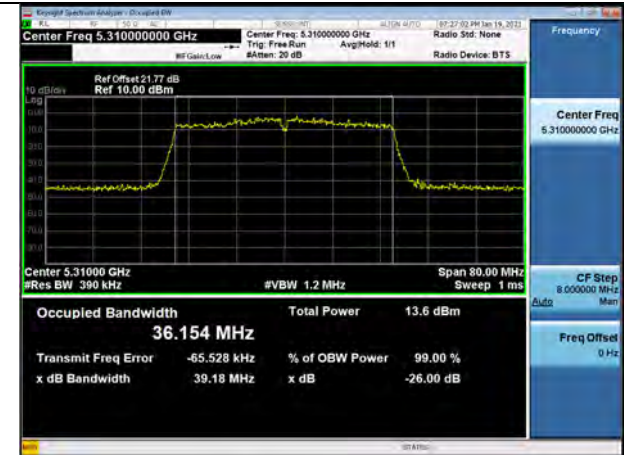
802.11ac_VHT40 UNII 3 BAND 26dB Bandwidth (CH 159)
