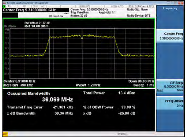
802.11n_HT40 UNII 3 BAND 26dB Bandwidth (CH 159)
