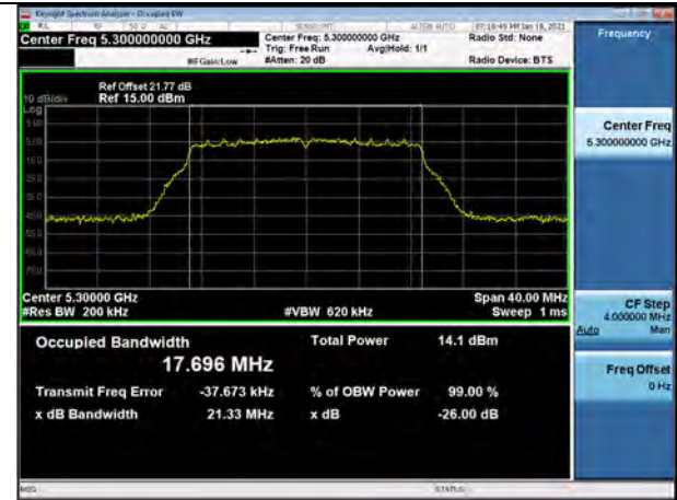
802.11ac_VHT20 UNII 3 BAND 26dB Bandwidth(CH 149)
