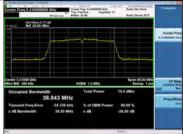
802.11n_HT40 UNII 3 BAND 26dB Bandwidth (CH 151)
