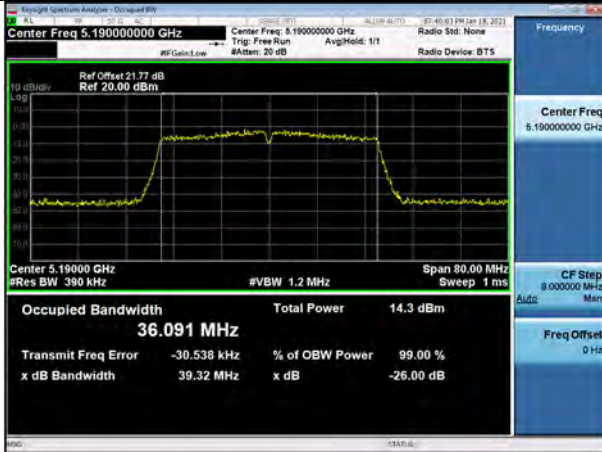
802.11n_HT40 UNII 2C BAND 26dB Bandwidth(CH 142)
