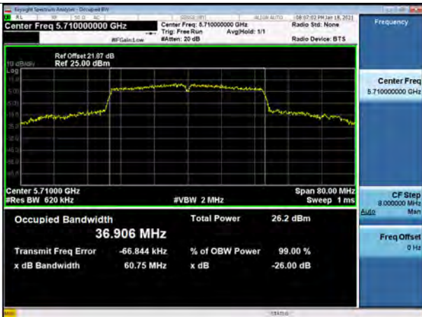
802.11ac_VHT40 UNII 2C BAND 26dB Bandwidth(CH 142)
