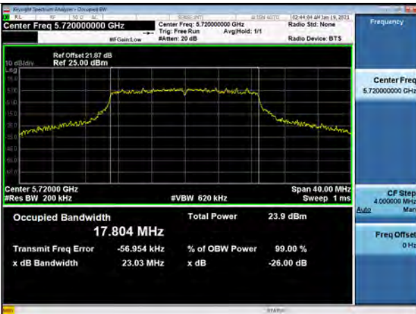
802.11n_HT20 UNII 2C BAND 26dB Bandwidth(CH 144)
