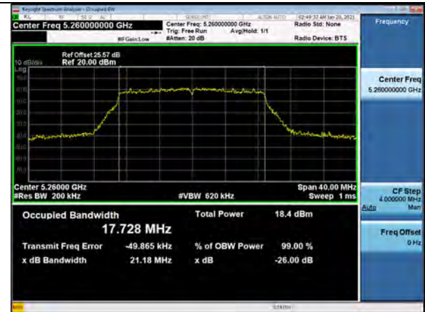
802.11n_HT20 UNII 3 BAND 26dB Bandwidth(CH 165)
