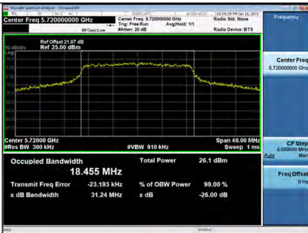
802.11n_HT20 UNII 2C BAND 26dB Bandwidth(CH 144)
