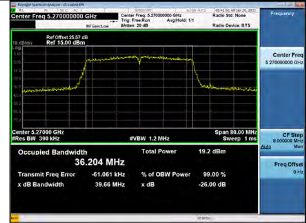
802.11ac_VHT40 UNII 3 BAND 26dB Bandwidth (CH 159)
