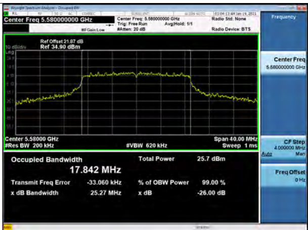
802.11ac_VHT20 UNII 2C BAND 26dB Bandwidth(CH 116)
