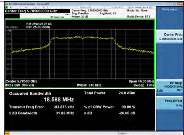
802.11n_HT20 UNII 3 BAND 26dB Bandwidth(CH 157)
