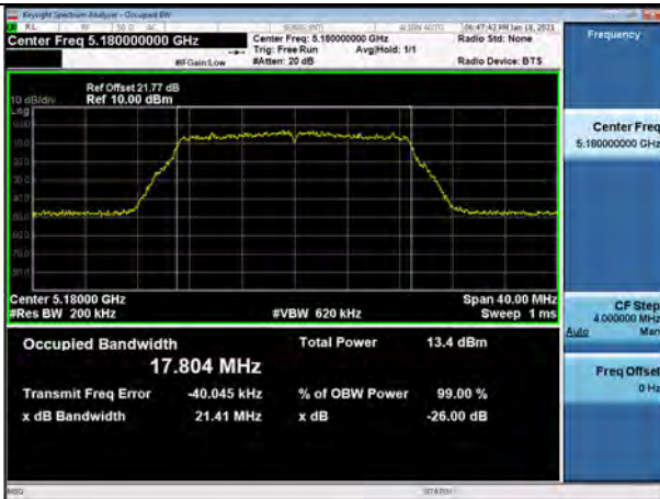
802.11n_HT20 UNII 2C BAND 26dB Bandwidth(CH 144)
