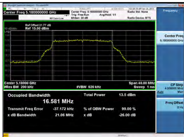
802.11a UNII 2C BAND 26dB Bandwidth (CH144)
