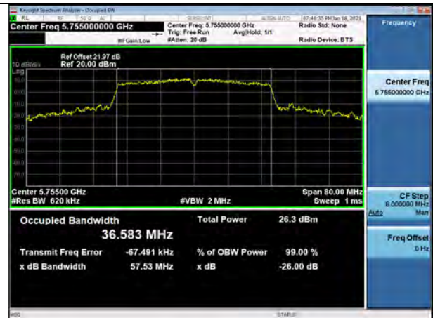
802.11n_HT40 UNII 3 BAND 26dB Bandwidth (CH 151)
