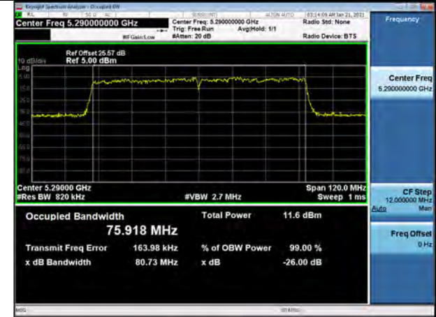
802.11ac_VHT80 UNII 3 BAND 26dB Bandwidth (CH 155)
