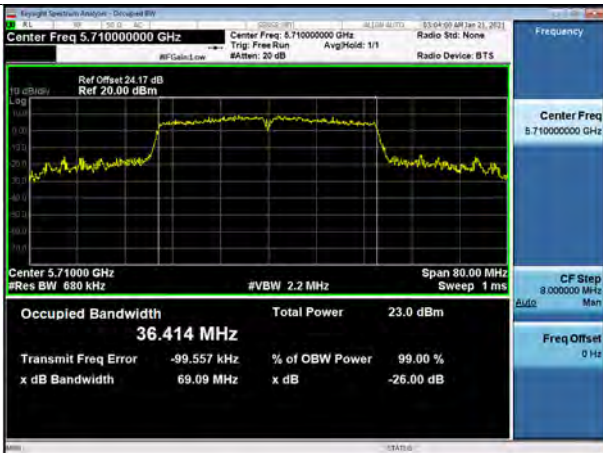
802.11ac_VHT40 UNII 2C BAND 26dB Bandwidth(CH 142)
