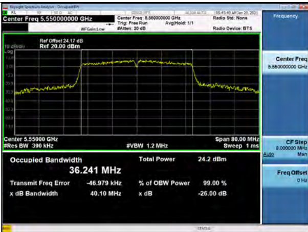
802.11ac_VHT40 UNII 2C BAND 26dB Bandwidth(CH 110)
