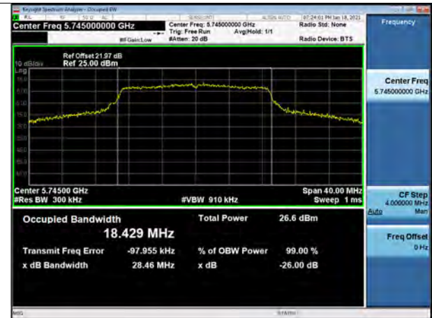
802.11ac_VHT20 UNII 3 BAND 26dB Bandwidth(CH 149)
