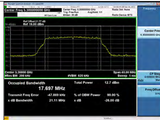
802.11ac_VHT20 UNII 3 BAND 26dB Bandwidth(CH 157)
