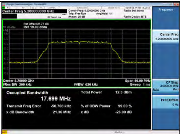
802.11ac_VHT20 UNII 2C BAND 26dB Bandwidth(CH 116)
