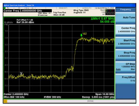
Test Plots with hopping ( $\pi$ /4DQPSK) Band Edges (CH.78)
