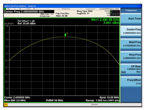
Test Plots (8DPSK) Peak Power (CH.0)
