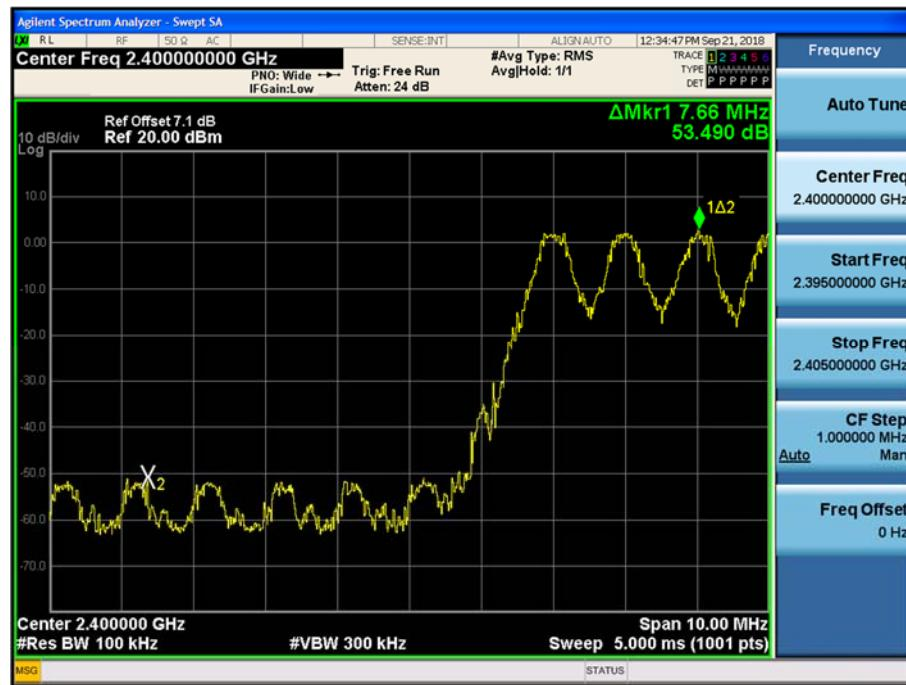
Test Plots with hopping (GFSK)
