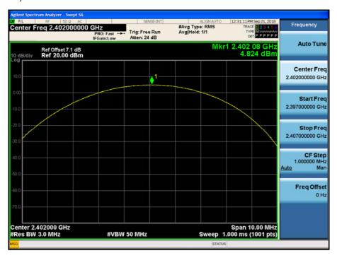
Test Plots (π/4DQPSK) Peak Power (CH.39)
