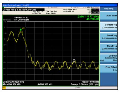
Test Plots with hopping (8DPSK) Band Edges (CH.0)
