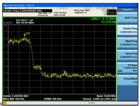
Test Plots with hopping ( $\pi$ /4DQPSK) Band Edges (CH.0)
