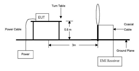
The diagram below shows the test setup that is utilized to make the measurements for emission from 30  $\,\mathrm{Mz}$  to 1  $\,\mathrm{Gz}$  emissions.
