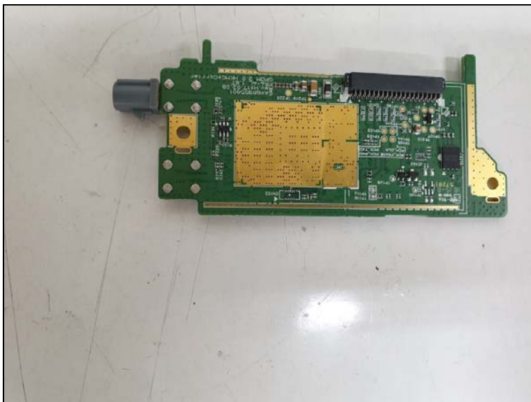
Bottom view of WWAN PCB
