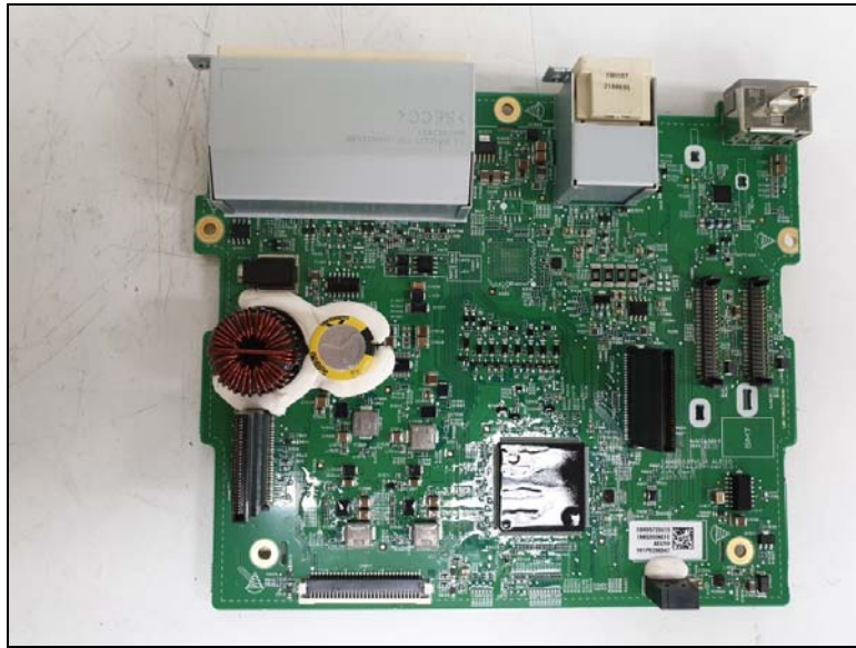
Top view of Main PCB
