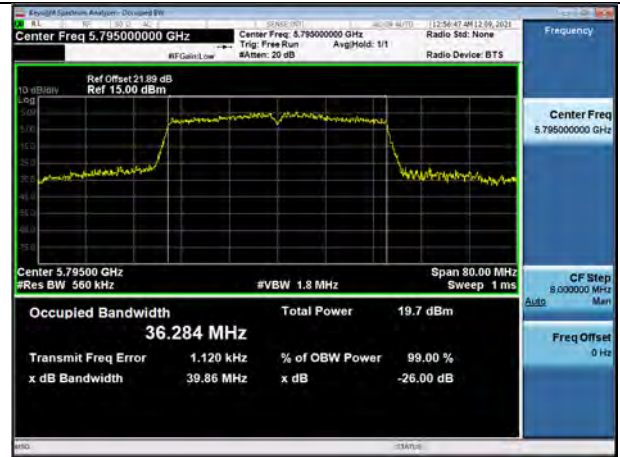
802.11ac_VHT40 UNII 3 BAND 26dB Bandwidth (CH 159)
