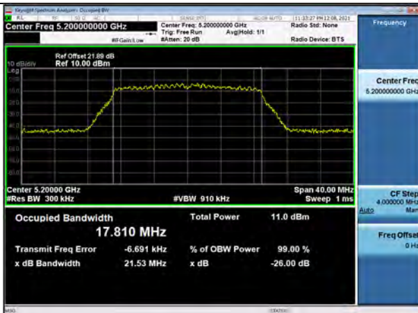
802.11n_HT20 UNII 1 BAND 26dB Bandwidth(CH 40)
