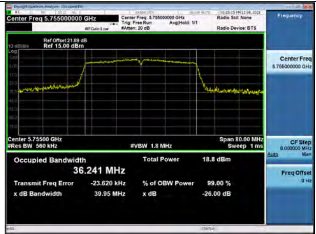
802.11ac_VHT40 UNII 3 BAND 26dB Bandwidth (CH 151)
