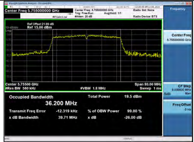
802.11n_HT40 UNII 3 BAND 26dB Bandwidth (CH 151)
