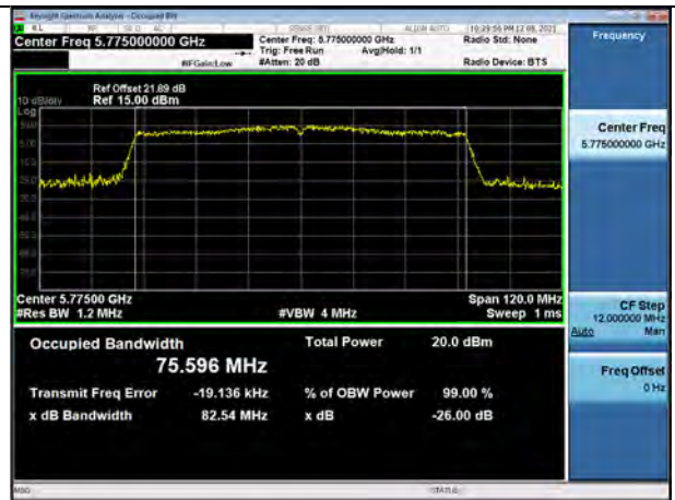
802.11ac_VHT80 UNII 3 BAND 26dB Bandwidth (CH 155)
