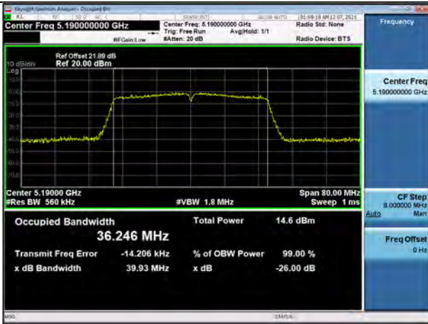
802.11ac_VHT40 UNII 1 BAND 26dB Bandwidth(CH 38)
