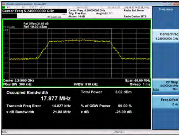
802.11ac_VHT20 UNII 1 BAND 26dB Bandwidth(CH 48)
