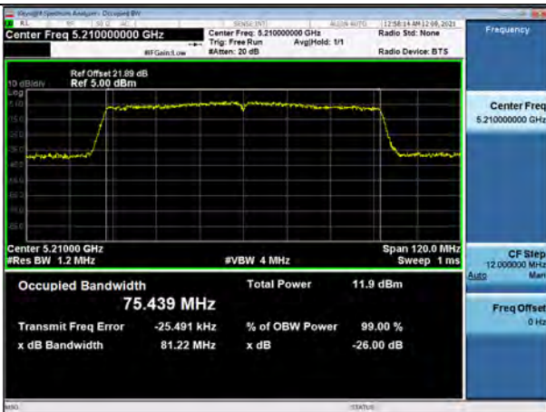
802.11ac_VHT80 UNII 1 BAND 26dB Bandwidth(CH 42)
