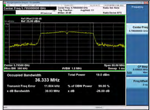
802.11n_HT40 UNII 3 BAND 26dB Bandwidth (CH 159)
