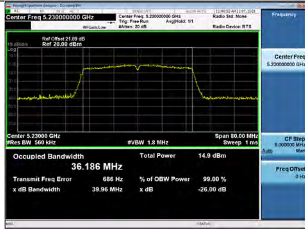
802.11n_HT40 UNII 1 BAND 26dB Bandwidth(CH 46)
