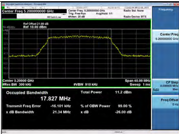
802.11ac_VHT20 UNII 1 BAND 26dB Bandwidth(CH 40)
