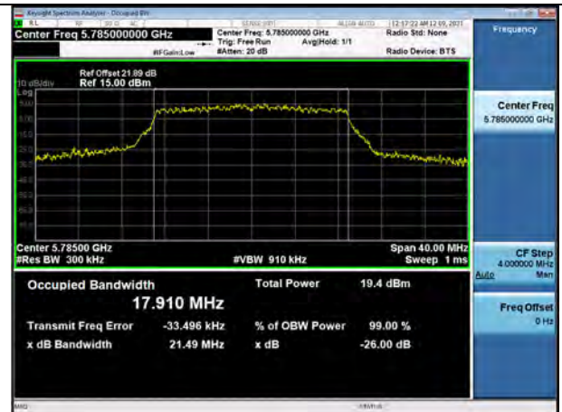
802.11ac_VHT20 UNII 3 BAND 26dB Bandwidth(CH 157)
