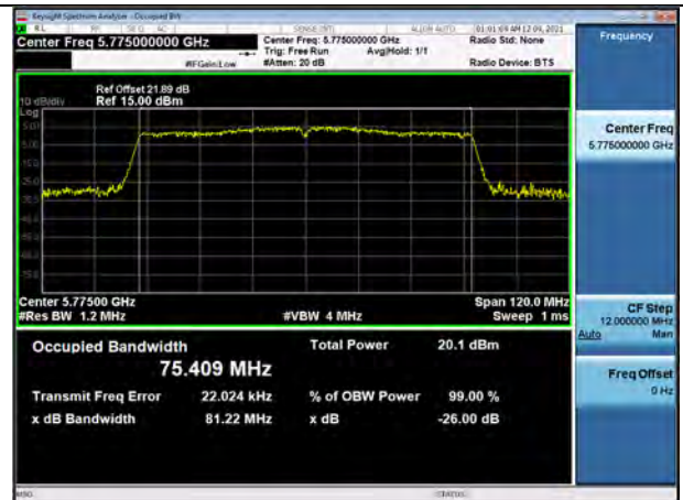
802.11ac_VHT80 UNII 3 BAND 26dB Bandwidth (CH 155)
