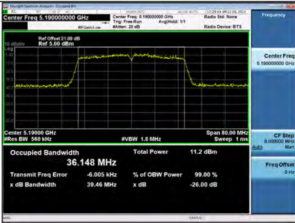
802.11ac_VHT40 UNII 1 BAND 26dB Bandwidth(CH 38)
