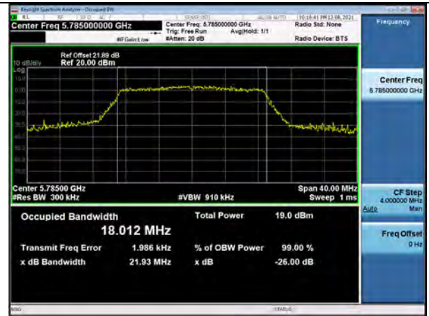
802.11ac_VHT20 UNII 3 BAND 26dB Bandwidth(CH 157)
