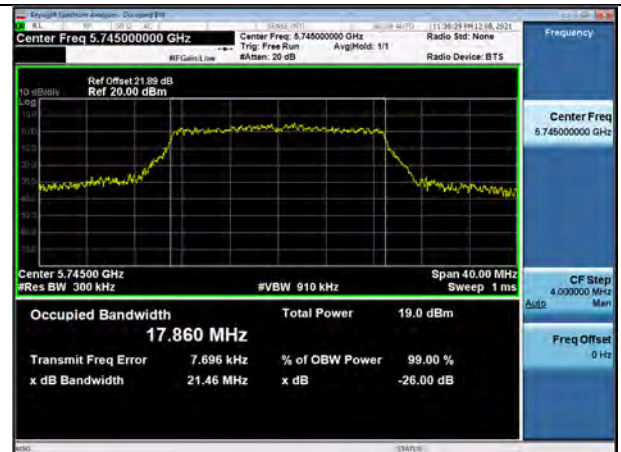
802.11n_HT20 UNII 3 BAND 26dB Bandwidth(CH 149)
