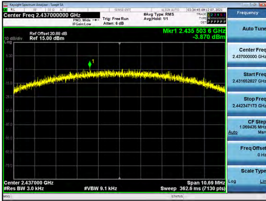
Power Spectral Density (802.11b-CH 6)
