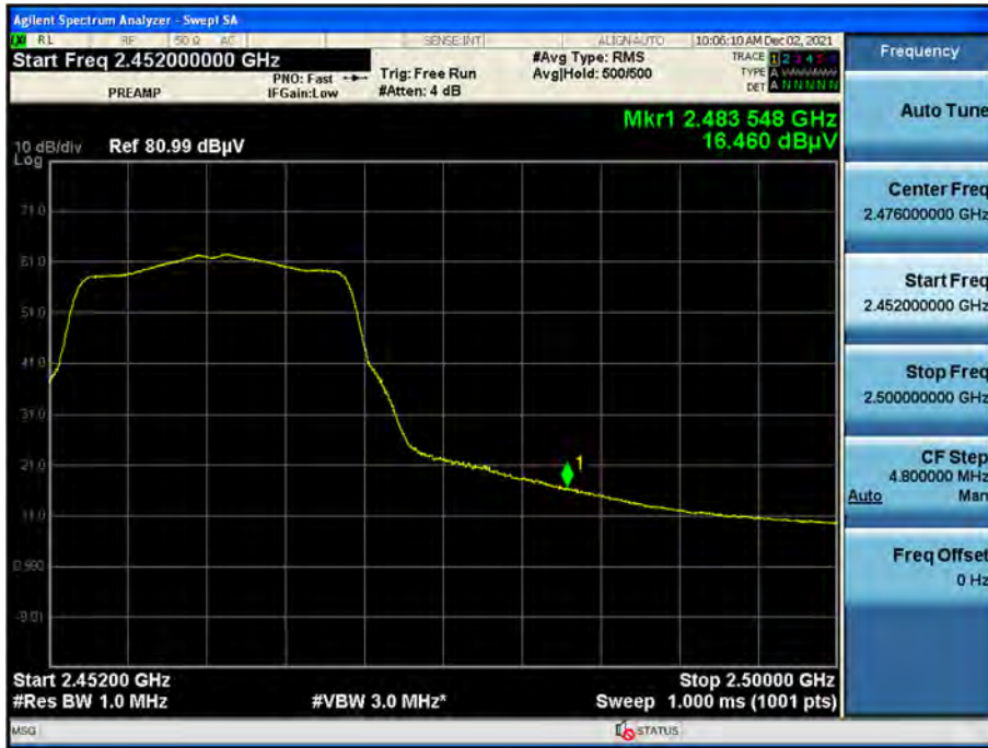
Radiated Restricted Band Edges plot – Peak Result (802.11g Ch.11, Y-V)
