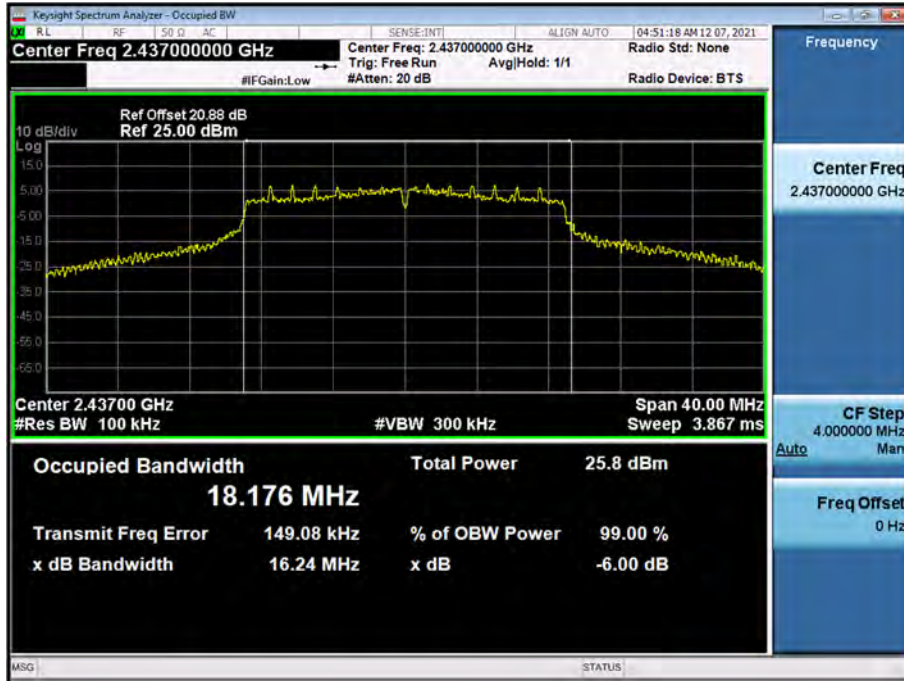
6 dB Bandwidth plot (802.11n_HT20-CH 6)
