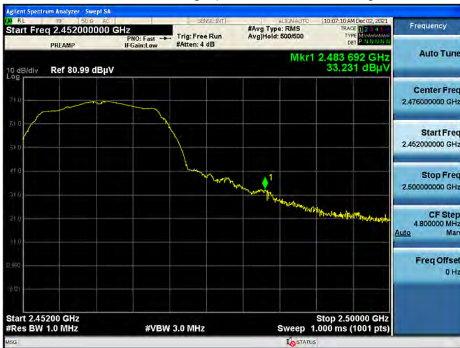
Radiated Restricted Band Edges plot – Peak Result (802.11g Ch.11, Y-V)
