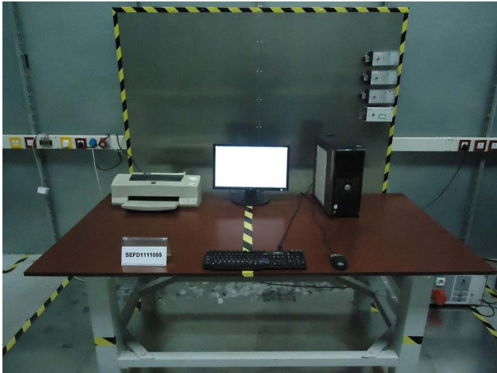
Front View of Conducted Emission Test
