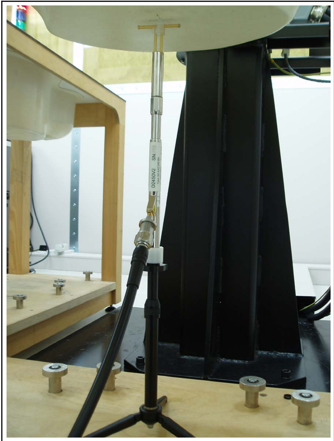
Figure 3 2450 MHz Dipole Validation Test Setup
