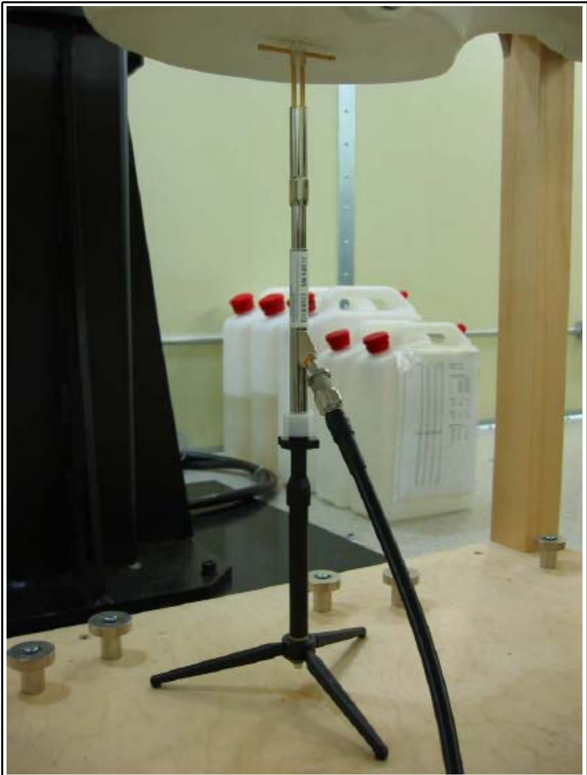
Figure 2 1900 MHz Dipole Validation Test Setup
