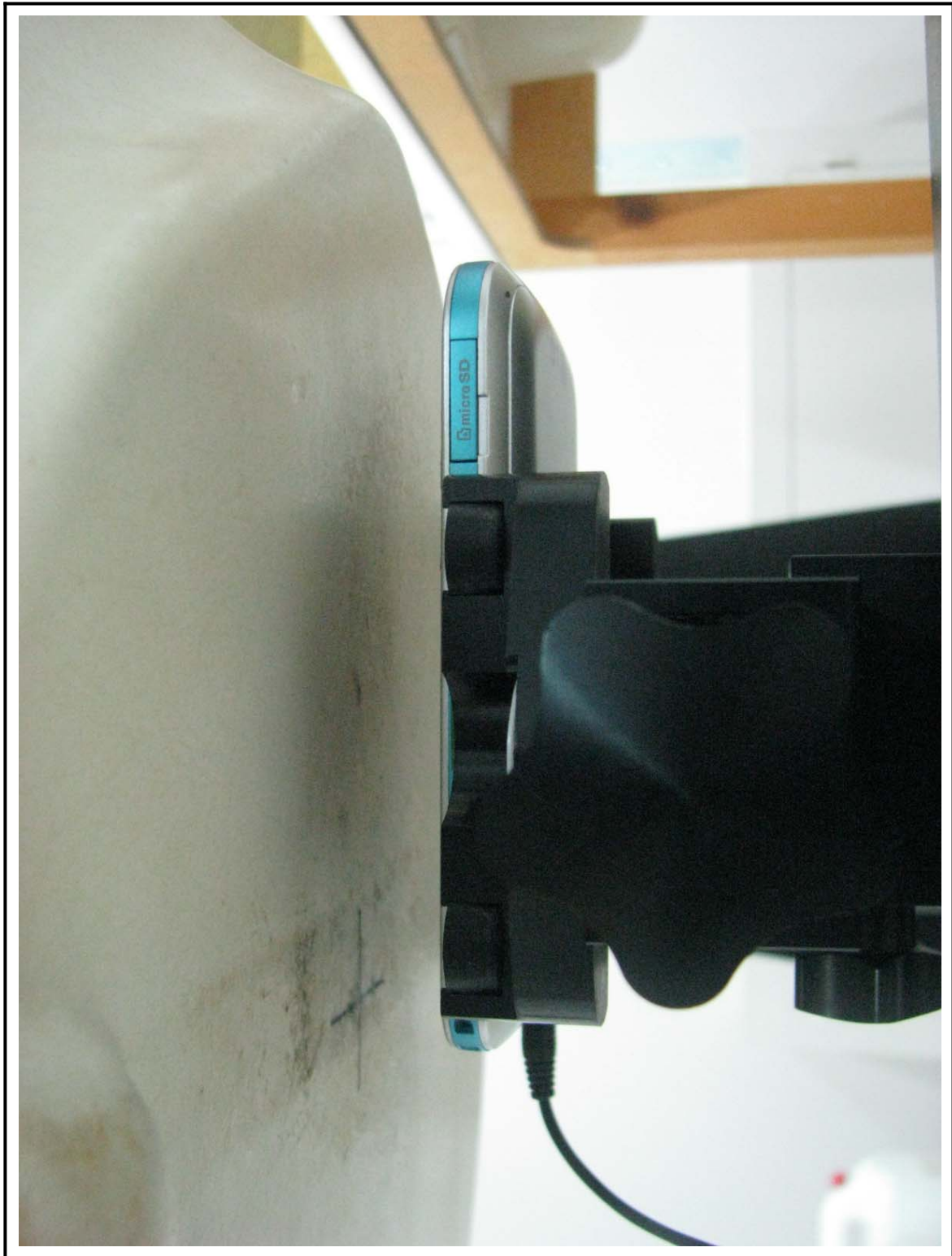
Figure 5 Body SAR Test Setup – w/o Holster
