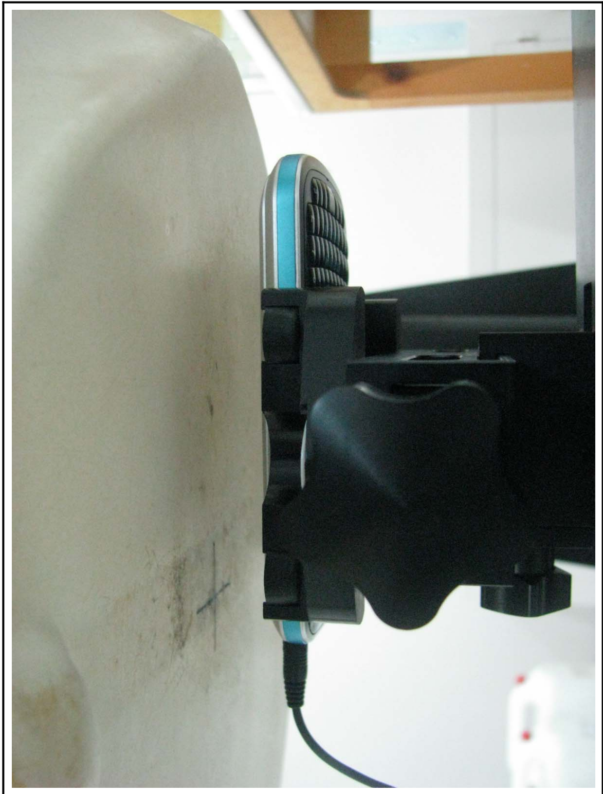
Figure 6 Body SAR Test Setup – w/o Holster
